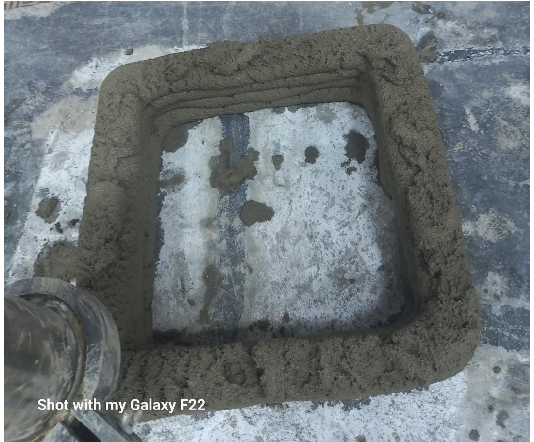
Figure 40 End of open time with interruption and rough surface of filaments after 2min of printing
