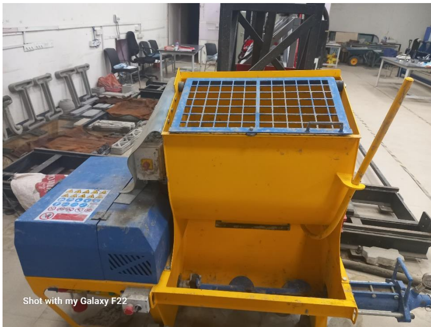
Figure 28 Pump integrated material mixer -3DCP. POD, IIT Indore.
