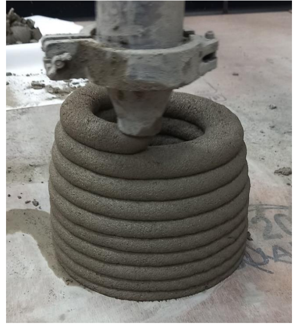
Figure 37 Illustrate image for Buildability- PASS (Smooth surface and continuous print)
