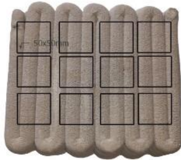
Figure 41 Cutting of slab into cubes- 50x50x50mm
