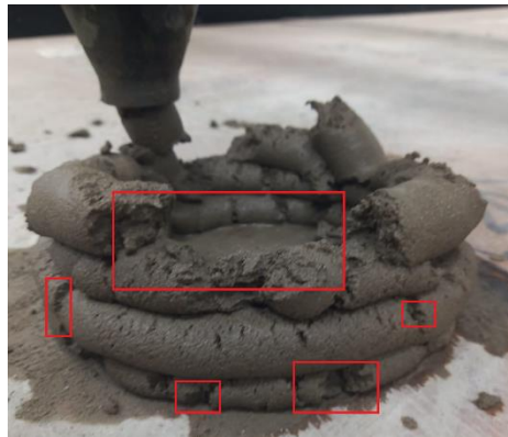
Figure 38 Illustrate image for Buildability- FAIL (Not Extrudable slump, Stiff)
