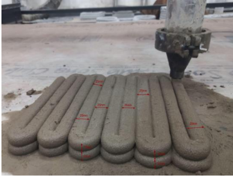
Figure 33 Illustrate Extrudability- PASS (Smooth surface and continuous print)
