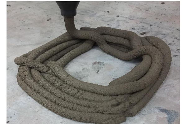
Figure 39 Illustrate image for Buildability- FAIL (Overflow and collapsible slump)
