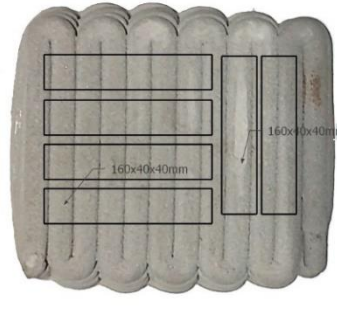
Figure 42 Cutting of slab in beam- 160x40x40mm
