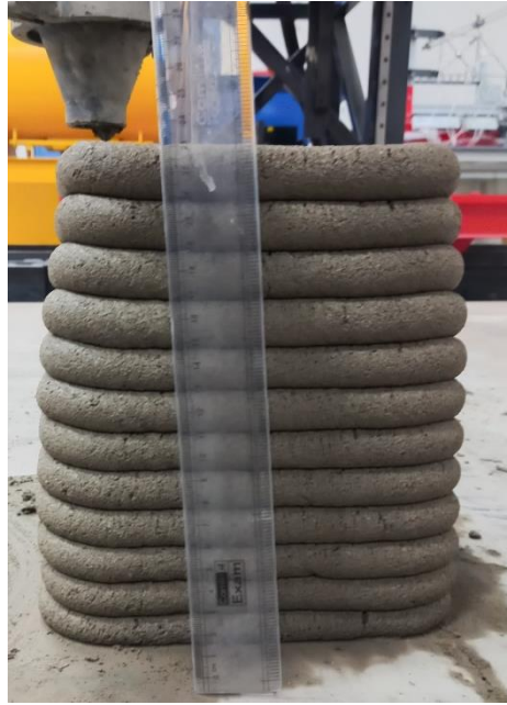
Figure 36 Illustrate image for Buildability- PASS (Smooth surface and continuous print)
