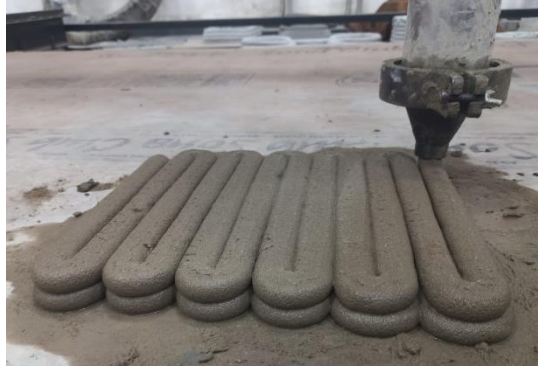
Figure 30 Extruded layers with uniform thickness and Height
