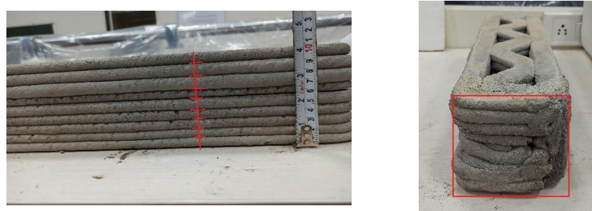
Figure 27 Inconsistent layer height
