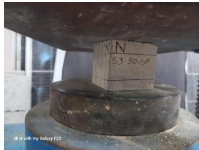
Figure 31 Compression testing of cube
