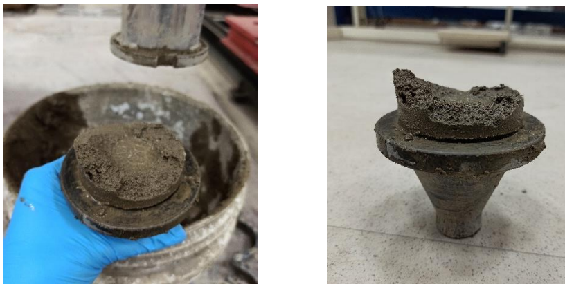
Figure 26 Material deposition and jamming of nozzle
