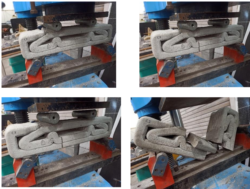
Figure 32 Crack formation and ultimate failure of topology optimized 3DCP beam
