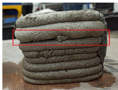
Figure 24 Delamination of layer
