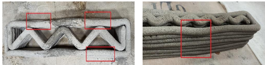
Figure 22 Layer misalignment in beam
