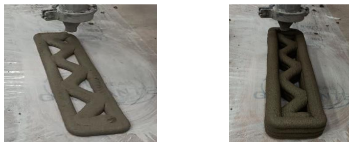
Figure 21 Printing of S-infill 3DCP beam
