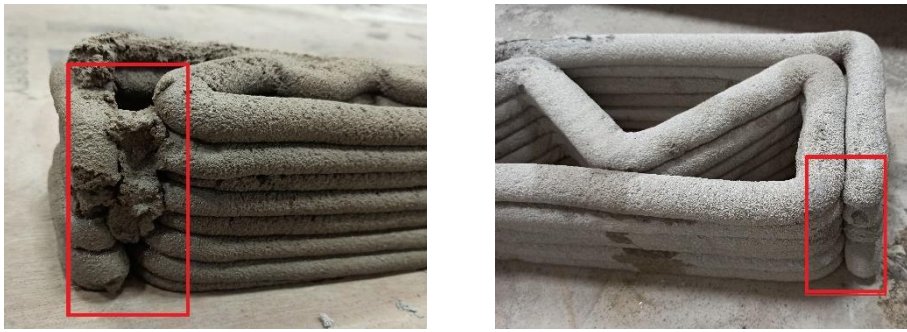
Figure 23 Initial extrusion delay defect
