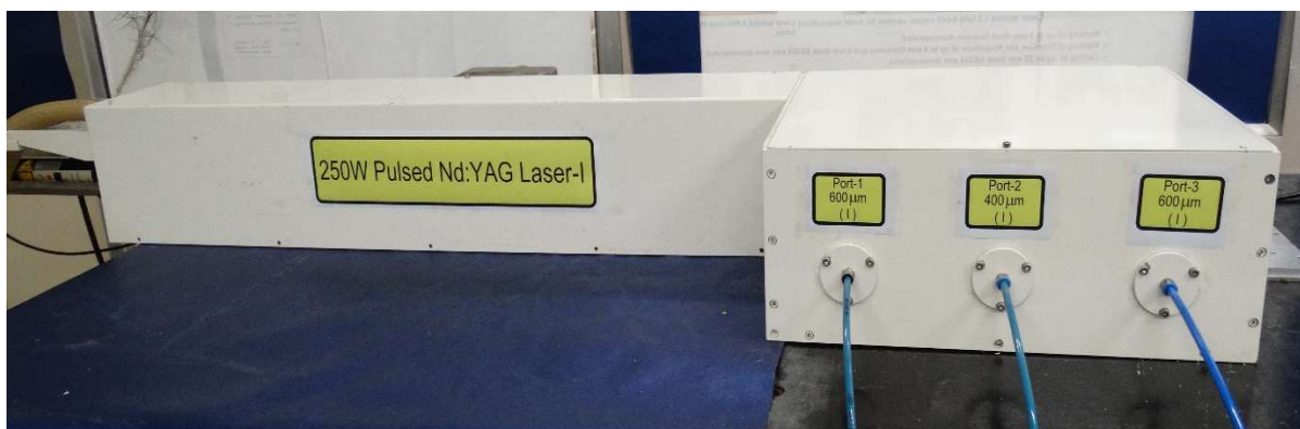
Fig. 3.5: 250 W average power and 5kW peak power industrial Nd: YAG laser with multi-port fiber optic beam delivery at RRCAT, Indore.
