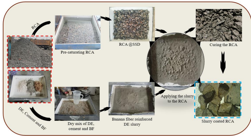
Figure 13 Treatment process of RCA
