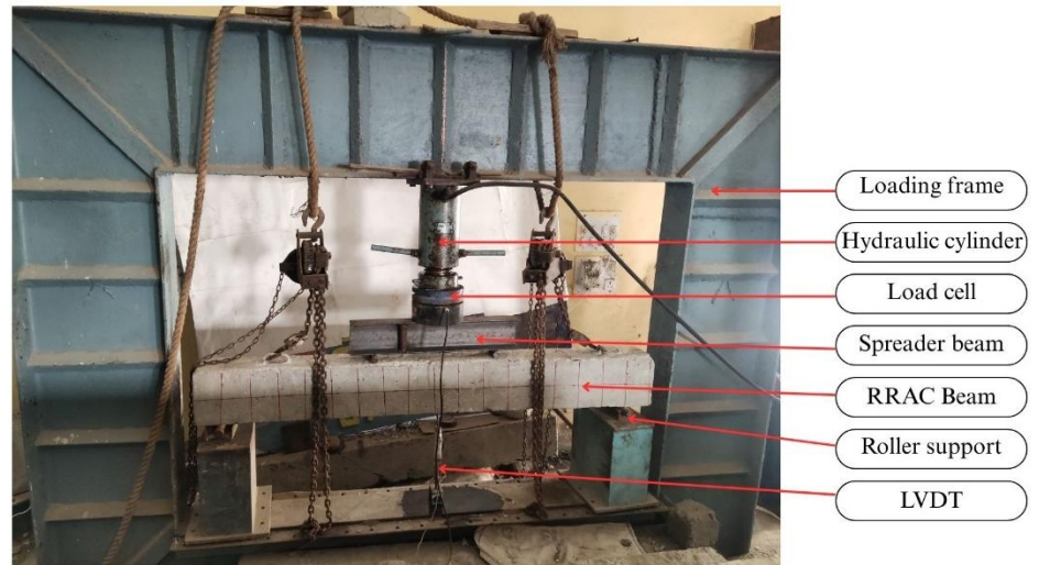
Figure 23 Four bending test setup
