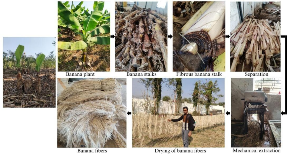
Figure 11 Mechanical extraction process of banana fiber
