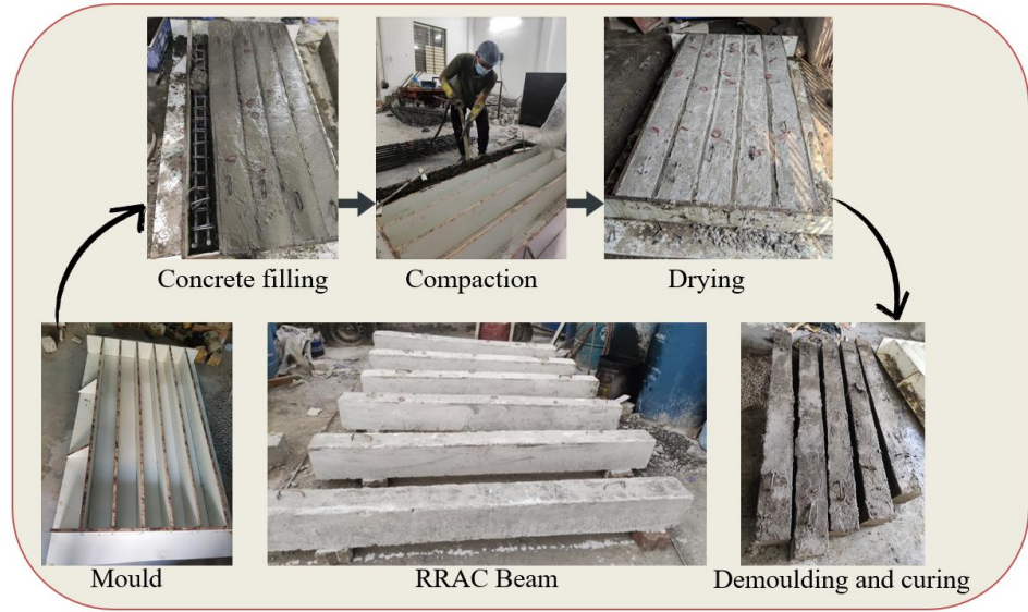
Figure 21 Casting of beam
