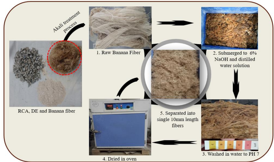
Figure 12 Treatment process of banana fiber
