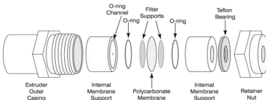
**Figure 1.3 : Extrusion apparatus- Assembly of extruder [27]**
