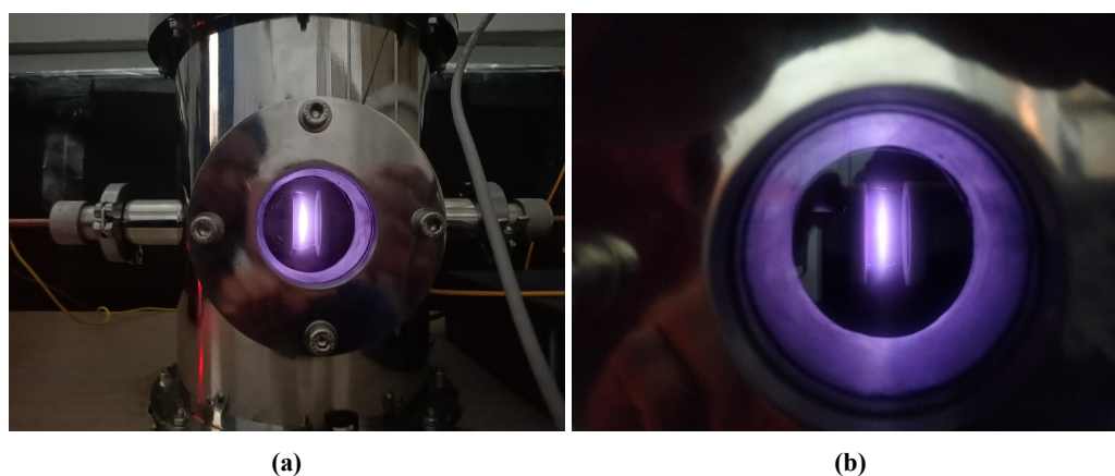
Figure 3.14: Plasma generation using (a.) air and (b.) argon as the working gases. The Teflon jackets insulating the rear side of the electrodes are also visible.
