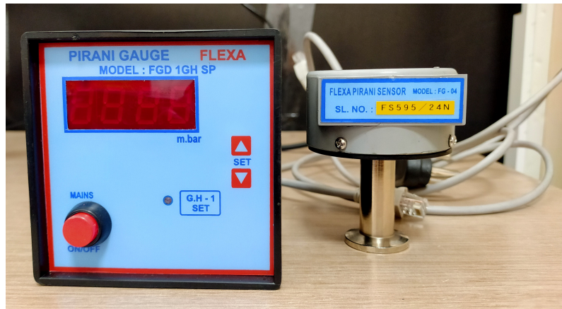
Figure 3.11: Pirani gauge & gauge head for pressure measurement.
