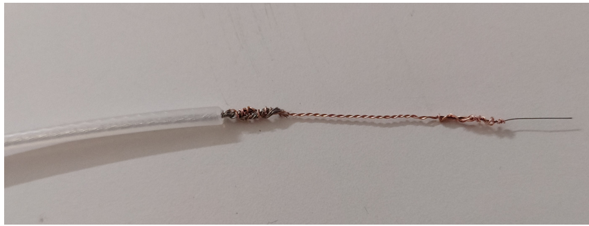
Figure 5.8: Threading of the tungsten probe tip with the 10 mm exposed aluminium conductor using thin copper wire.
