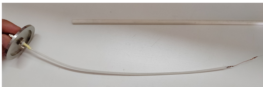
Figure 5.11: Fully assembled probe with BNC connector, prior to insertion into the ceramic insulation tube.
