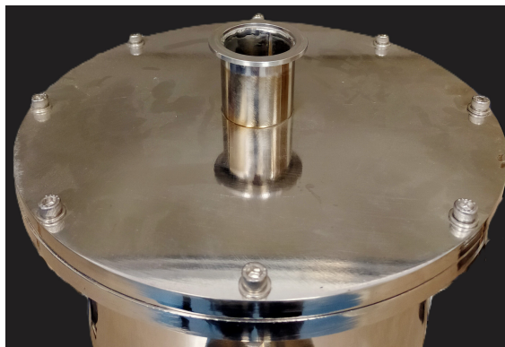
Figure 3.3: Top adapter flange with a 40 KF port for Tee configuration.
