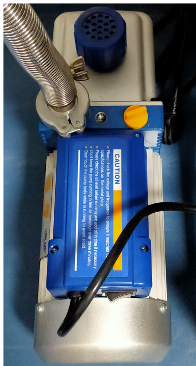
Figure 3.10: Vacuum pump setup with a vacuum hose for connection to the plasma chamber.
