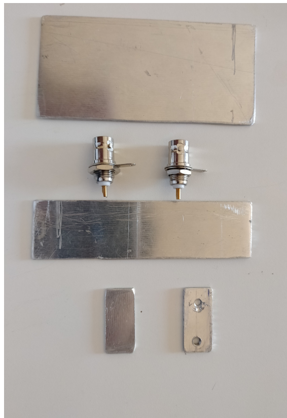
Figure 5.13: Raw materials for constructing the electronic circuit box: two aluminum sheets (pre-cut to required dimensions) and two panel-mount BNC connectors.
