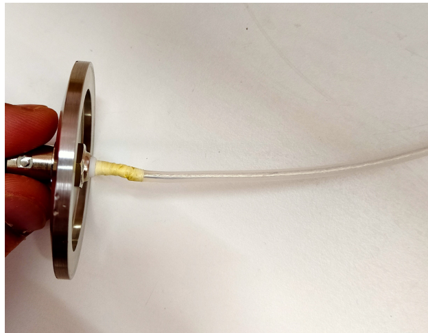
Figure 5.10: Soldering of the 5 mm exposed aluminum conductor to the female end of the BNC connector, followed by Teflon taping for mechanical stability and insulation.
