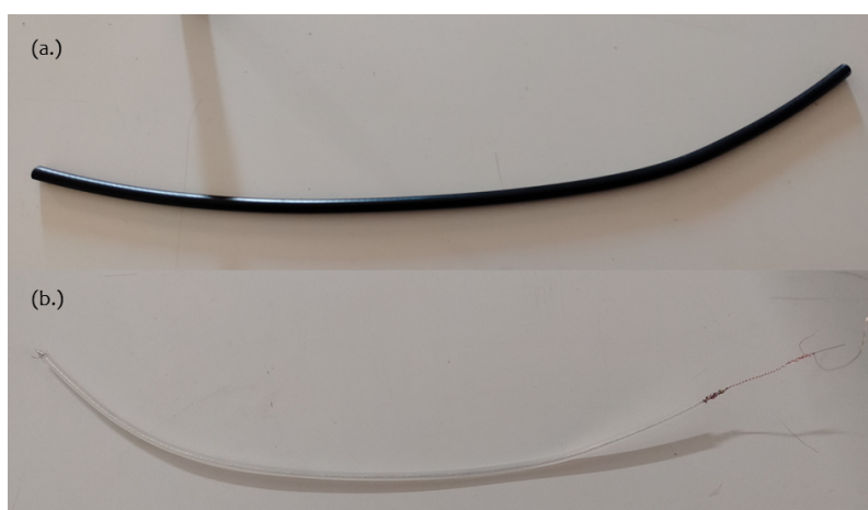
Figure 5.7: (a) 300 mm long coaxial cable used as the structural base for the Langmuir probe assembly; (b) Coaxial cable with outer insulation removed and both ends stripped to expose the internal aluminum conductor for electrical connections.
