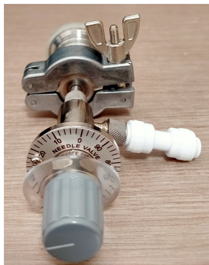
Figure 3.9: Needle valve to regulate argon gas flow through the chamber.
