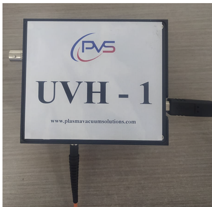
Figure 4.1: OES spectrometer featuring a camera sensor module designed for probing across the Ultraviolet (UV), Optical, and Infrared (IR) bands with a minimum resolution of 0.197nm.
