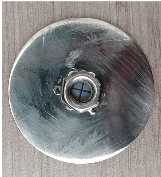
Figure 3.6: Electrode with Nut to Affix it to the High-Voltage Power Rod.
