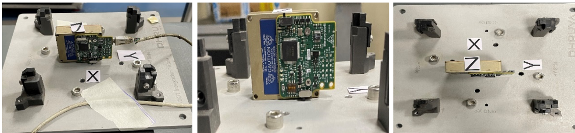
Figure 11: Position of IMU on the turntable (a) Front View (b) Isometric View (c) Top View
