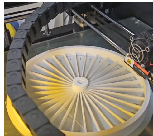
Figure 78: Lower hemispherical part being printed in 3D printing Machine.
