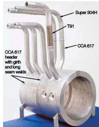
Fig. 1.7: Outlet header used in thermal power plants[18].
