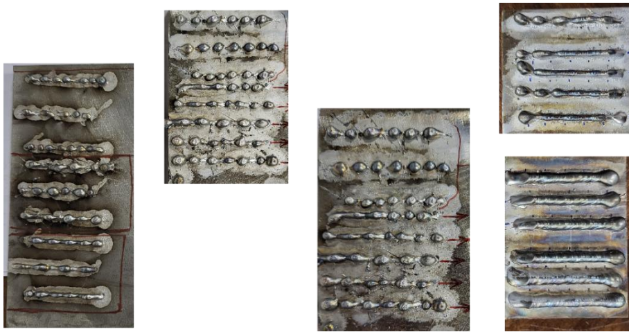
Fig. 4.7: Pilot experiments for optimizing the process parameters of WAAM
