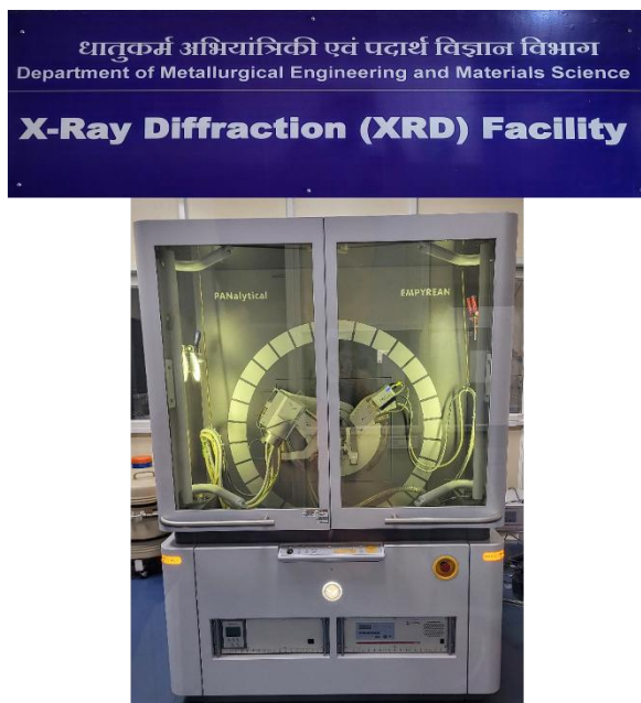
Fig. 3.10: X-ray diffractometer using Cu-K \alpha radiations
