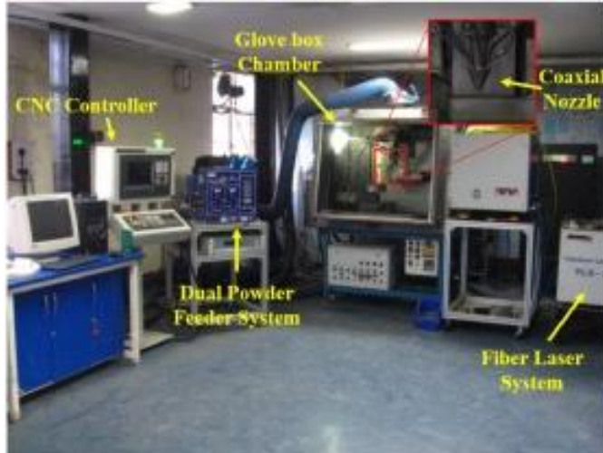
Fig. 3.1: 5-axis LAM-DED developed at RRCAT
