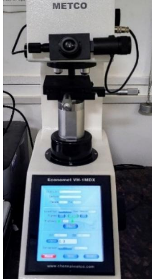
Fig. 3.12: Vickers microhardness test setup
