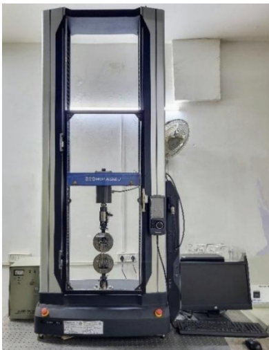
Fig. 3.13: Universal testing machine (left) and 2-D drawing for micro- tensile sample(right)
