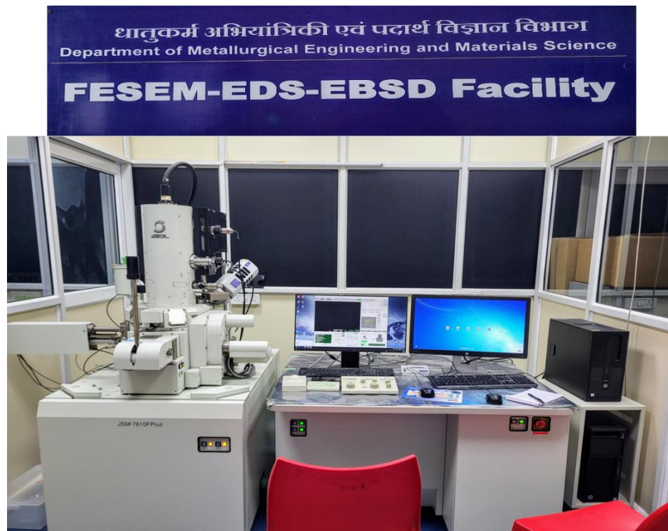
Fig. 3.9: Field Emission Scanning Electron Microscopy (FESEM)
