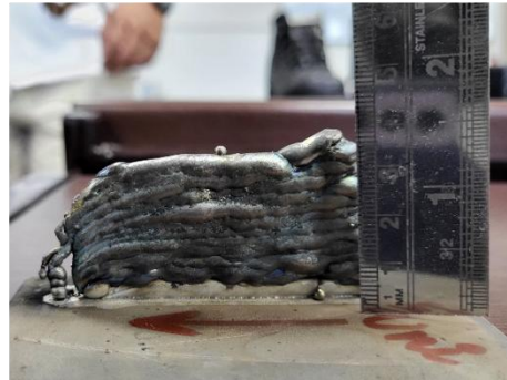
Fig. 4.20: Unidirectional deposition strategy schematic(left) and deposited wall(right)
