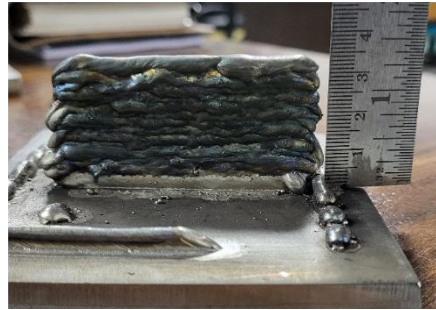
Fig. 4.19: Bidirectional deposition strategy schematic(left) and deposited wall(right)
