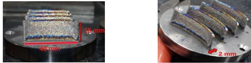
Fig 3.2 Deposition of blade height 15 mm with different power from 400 to 360 W
