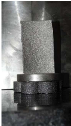
Fig 3.7 Deposited Profile Blade Ti6Al4V using DED
