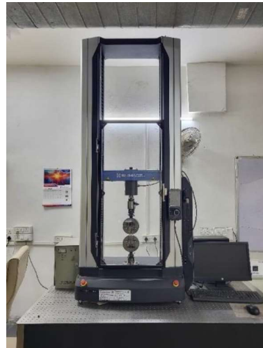
Fig. 2.6 Pictorial View of Compressive Strength Measurement Setup
