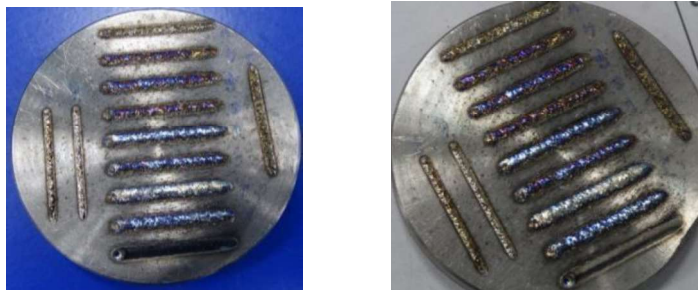
Fig 3.1 Track deposition on Titanium Plate
