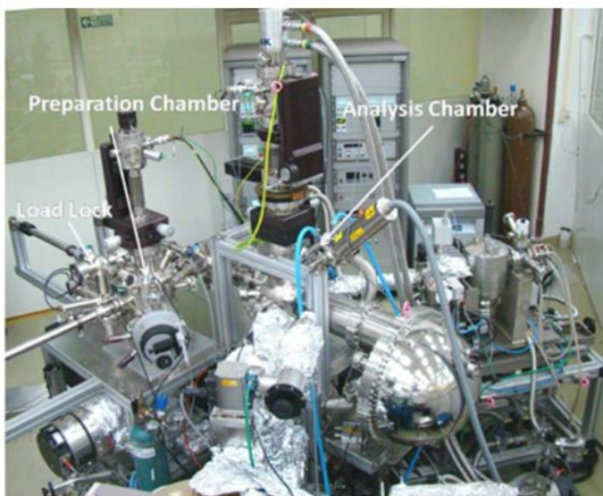
Figure 2.16: Instrumentation of the PES in Beamline 10, Indus II synchrotron facility [102].
