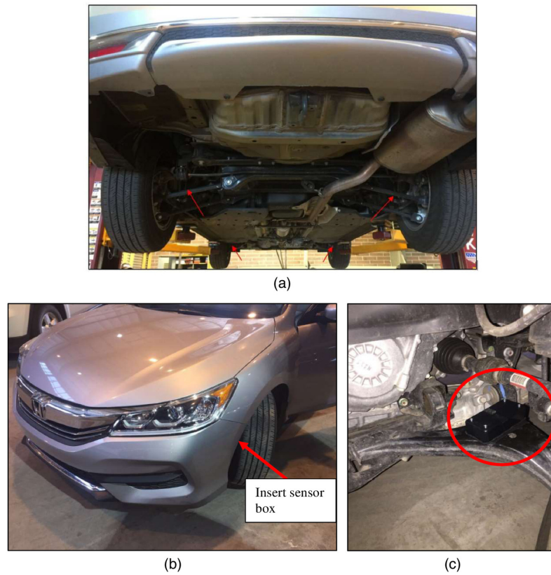
Figure 2.3: Accelerometer placement on vehicle: (a) overview of sensor installations; (b) direction of sensor box installation; and (c) placement of sensor box [3]
