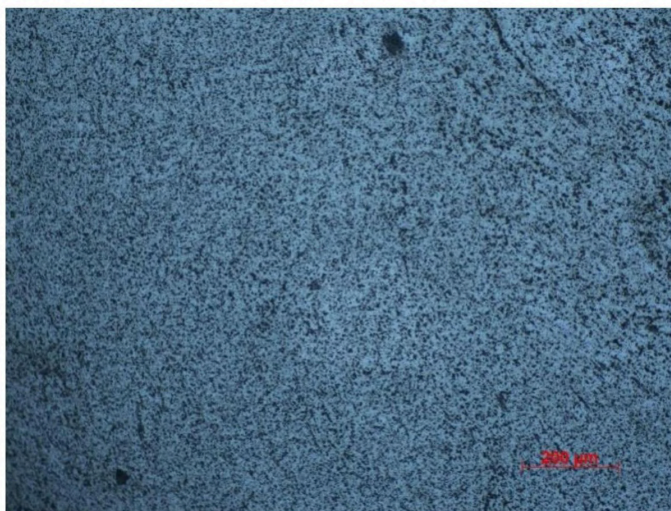
Figure 5.21: Microstructure of Side Longitudinal HPT (1 Turn) – Edge
