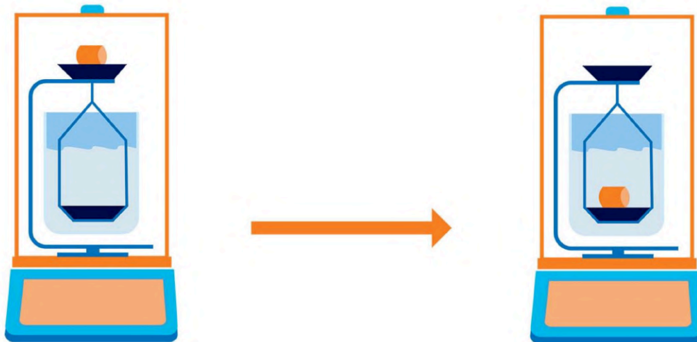
Figure 4.4: Systematic diagram of Archimedes Density Test
