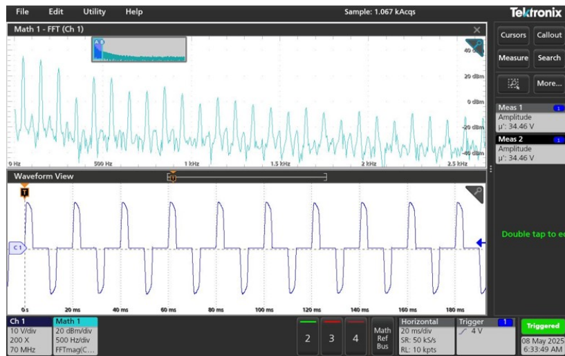
Figure 6.3: THD analysis of Diode Bridge Rectifier
