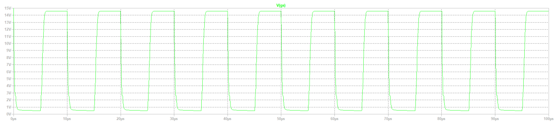
Figure 3.4: Simulation Output Showing V_{GS} of MOSFET
