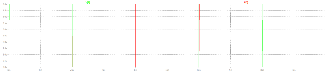
Figure 3.2: LTspice Simulation Waveform Showing Dead Band Delay
