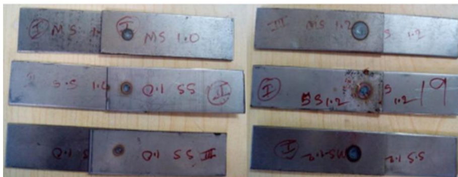
Figure 8 Spot welded mild steel and stainless-steel metal sheets [4]
