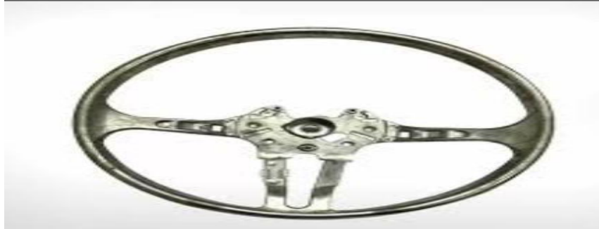
Fig1.2: Shows the real world use of Mg based alloys in fabricating steering wheels.
