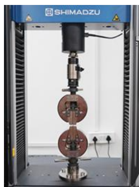
Fig. 3.4: UTM Setup for Tensile Test.
