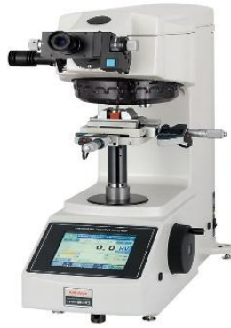
Fig. 3.8: Vicker Hardness Test Setup.
