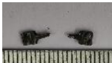
Fig 3.7: Tensile Sample After Failure.
