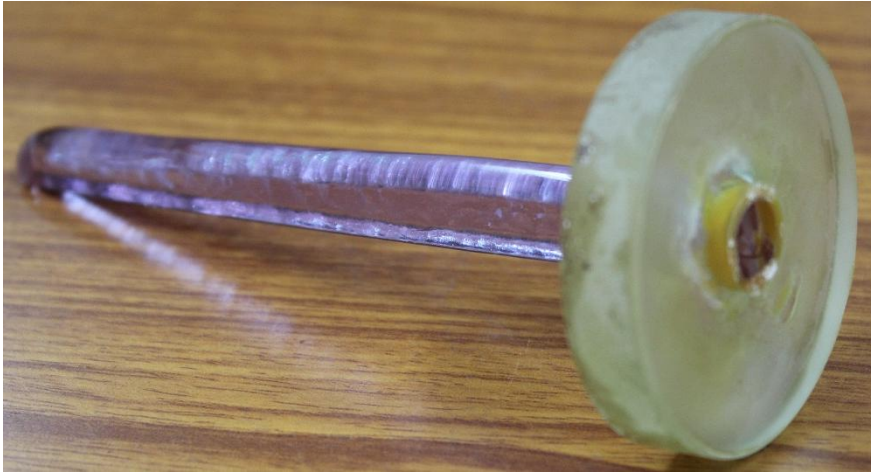
Fig. 5.5: Nd-glass rod holder used for polishing.
