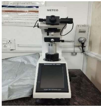
Fig:3.9 computer attached automated Vickers hardness machine
