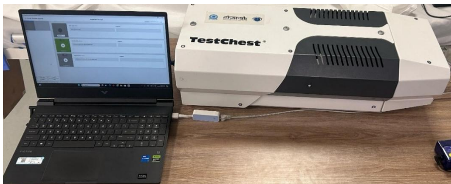
Figure 17 Testchest used for leakage simulation
