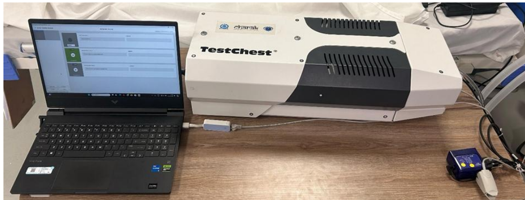
Figure 18 Testchest used for leakage simulation
