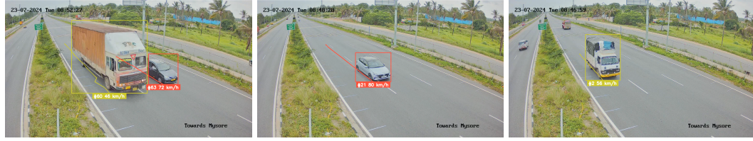
Figure 5.7: Real-time speed detection output showing vehicle bounding box, and estimated speed
