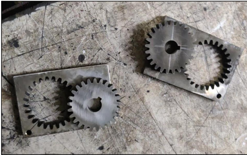
Figure 11 Gears manufactured using wire EDM.
