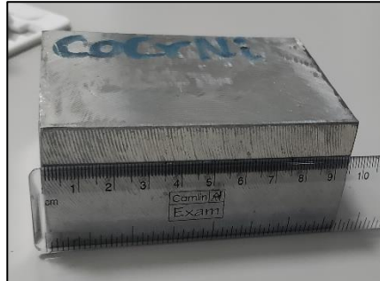
Figure 7 As-cast ingot of CoCrNi.
