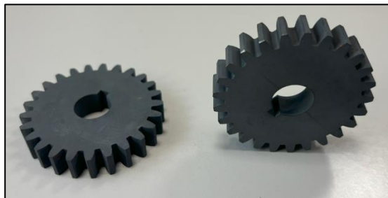
Figure 12 Gears post heat treatment at 1000°C in an Argon based environment.
