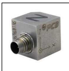
Figure 15 Triaxial accelerometer (225948) by PCB Piezotronics with sensitivities (in mV/g) in X, Y, and Z axes 50.3, 47.6, and 47.8 respectively.
