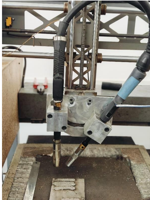
Fig. 3.10 Twin torch setup designed for Cu addition
