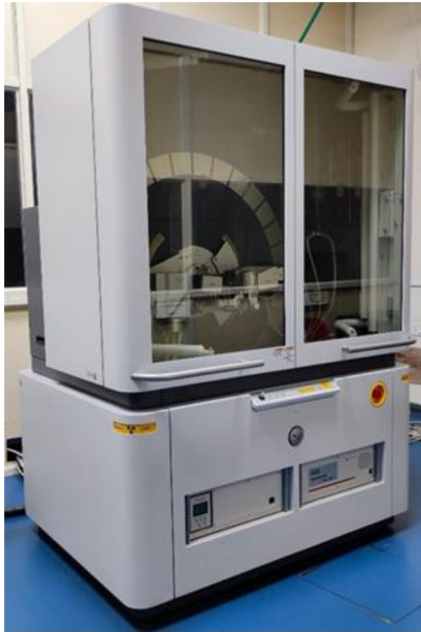
Fig. 3.5 X-ray diffractometer using Cu-K \alpha radiation.
