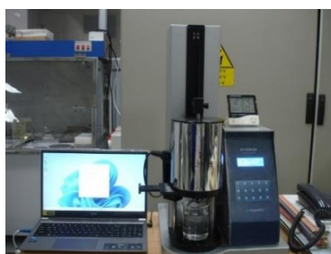
Fig.3 A dip coating unit used in the deposition. Fig. 4-Film deposition mechanism in dip coating.
