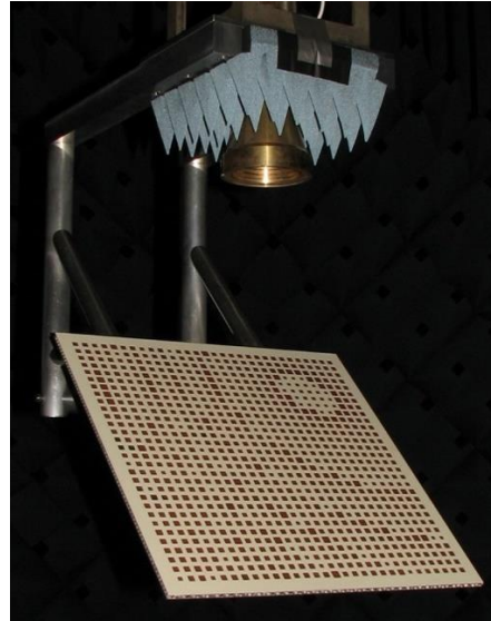
Figure 2.1: Reflectarray Setup [Ref. Wikipedia]
