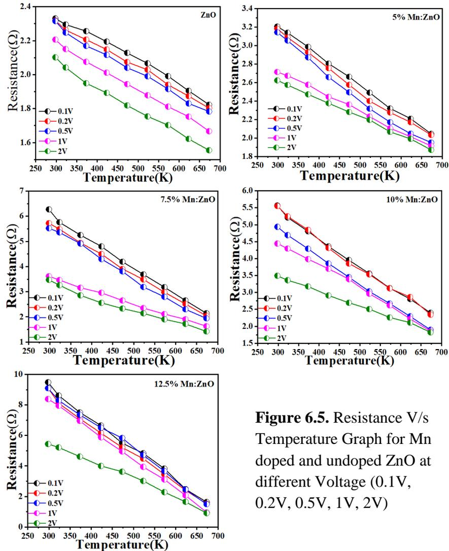
**Figure 6.5.** Resistance V/s Temperature Graph for Mn doped and undoped ZnO at different Voltage (0.1V, 0.2V, 0.5V, 1V, 2V)
