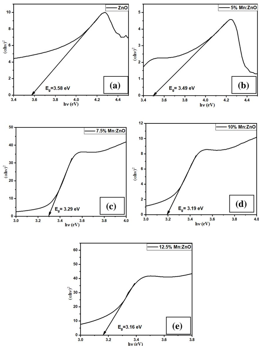
**Figure 5.8.** Band gap of (a) undoped ZnO (b) 5% Mn: ZnO (c) 7.5% Mn: ZnO (d) 10% Mn: ZnO (e) 12.5% Mn: ZnO
