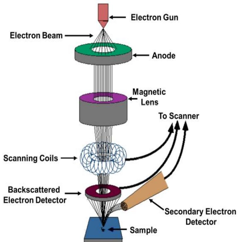
**Figure 3.3.** Schematic arrangement of FESEM[35]
