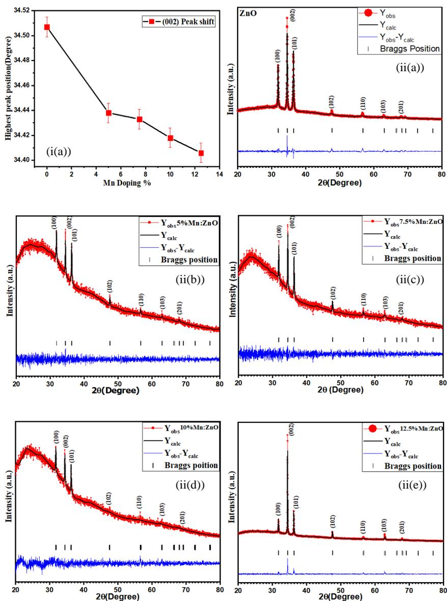
**Figure 5.4.** (i) Variation of (002) peak with Mn doping (ii) Rietveld Refinement XRD pattern of (a) undoped ZnO (b) 5%Mn: ZnO (c) 7.5%Mn: ZnO (d)10%Mn:ZnO (e) 12.5%Mn: ZnO.
