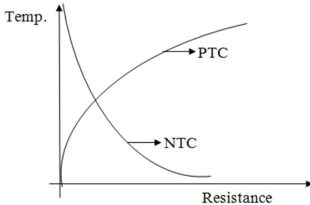
**Figure 6.1.** Temperature V/s Resistance graph for thermistors
