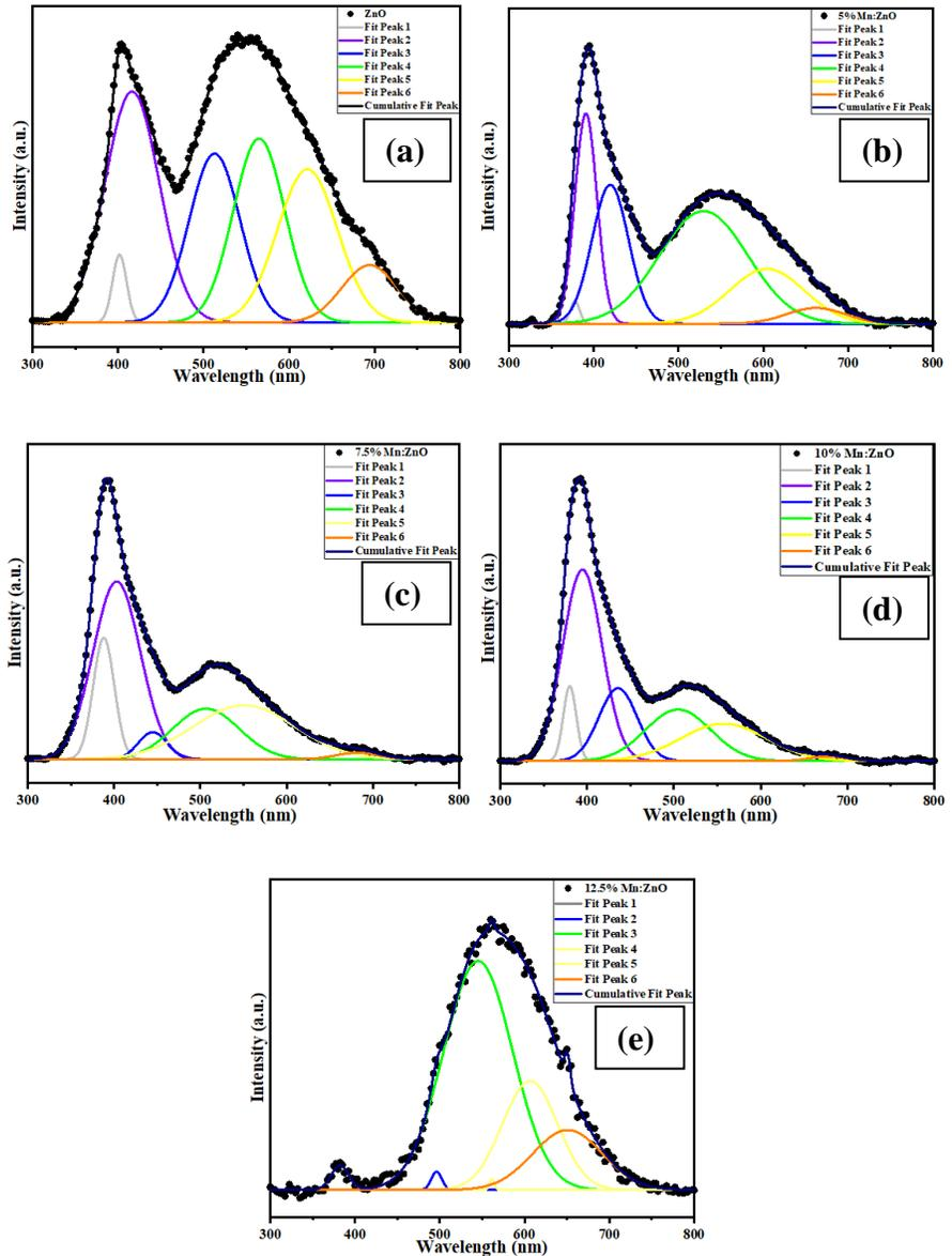
**Figure 5.11.** Fitted PL spectra of (a) undoped ZnO (b) 5%Mn: ZnO (c) 7.5%Mn: ZnO (d) 10%Mn: ZnO (e) 12.5%Mn: ZnO.
