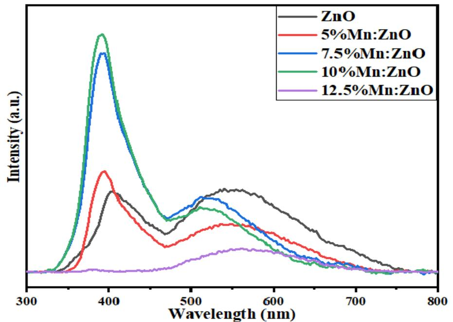
**Figure 5.9.** PL spectra of Mn doped and Undoped ZnO
