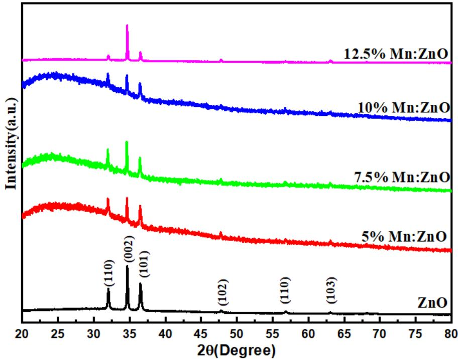
**Figure 5.3.** XRD pattern of Mn doped and undoped ZnO
