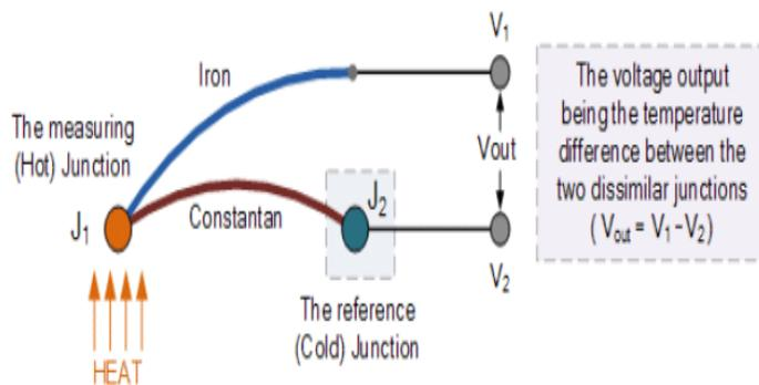
**Figure 6.2.** Setup of Thermocouple
