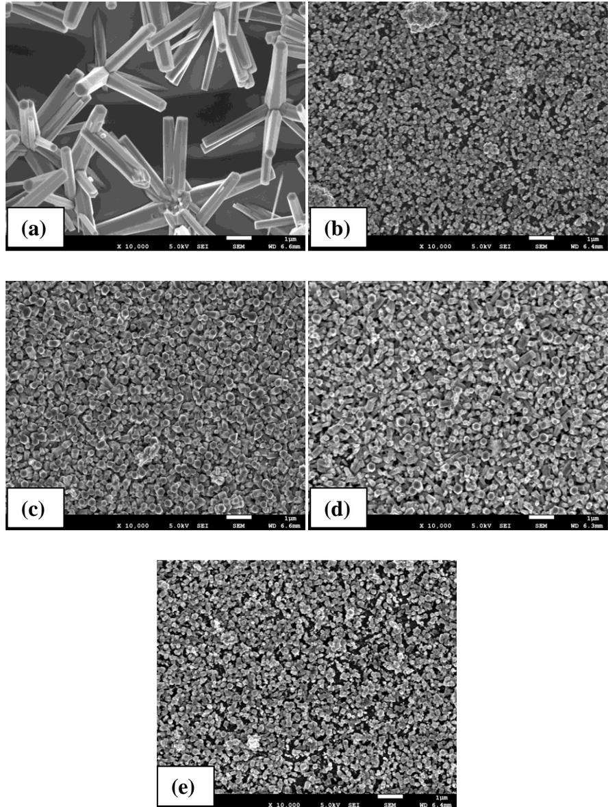
**Figure 5.2.** FESEM images at 10KX and scale 1 μm of (a) undoped ZnO (b) 5% Mn: ZnO (c) 7.5% Mn: ZnO (d) 10% Mn: ZnO (e) 12.5% Mn: ZnO.
