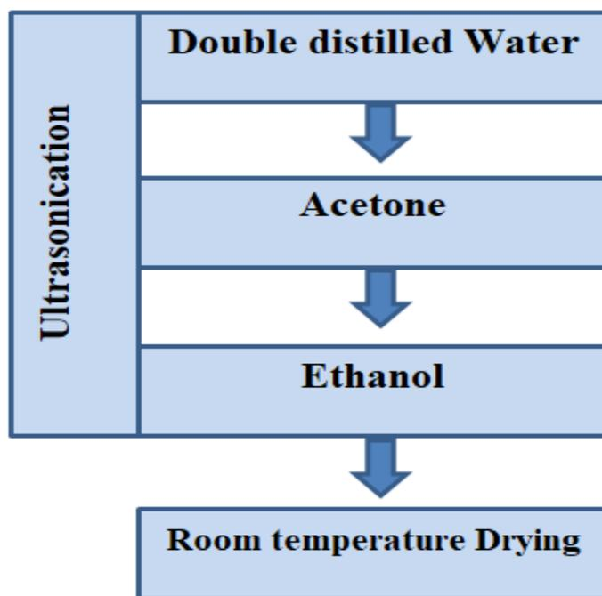
**Figure 4.1.** Procedure for substrate cleaning.
