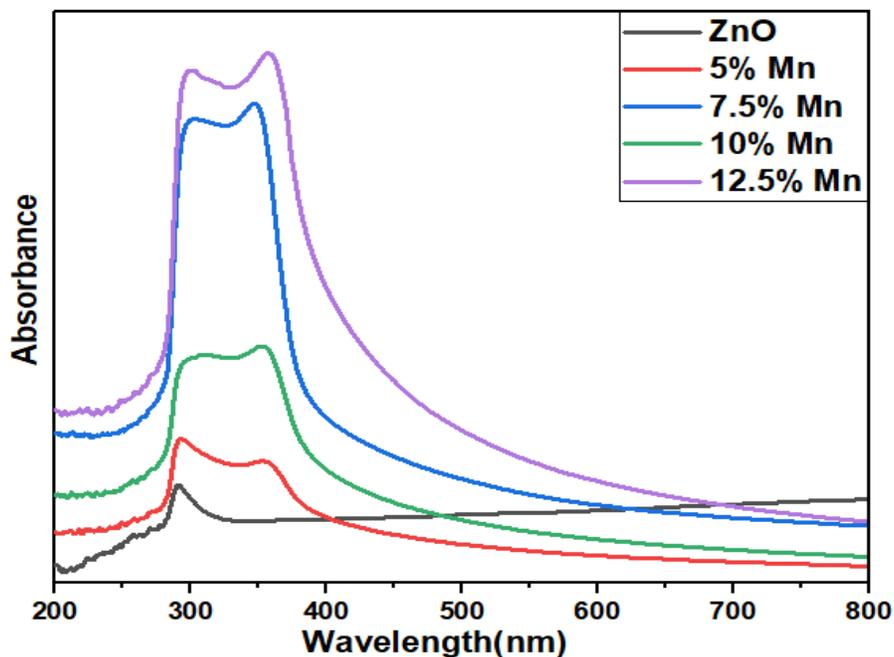
**Figure 5.7.** Room temperature UV-Visible spectra of Mn doped and undoped ZnO
