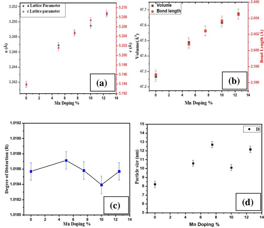
**Figure 5.5.** (a) Variation of lattice parameter ( $a$  &  $c$ ), (b) Variation of unit cell volume ( $V$ ) and Bond Length ( $L$ ), (c) Variation of Degree of Distortion, and (d) Variation of Particle size, with Mn doping %.
