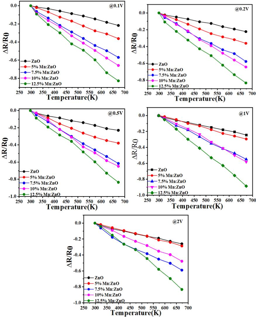
**Figure 6.6.** Relative change in resistance V/s Temperature graph of Pure and Mn doped ZnO at different Voltage (0.1V, 0.2V, 0.5V, 1V, 2V)
