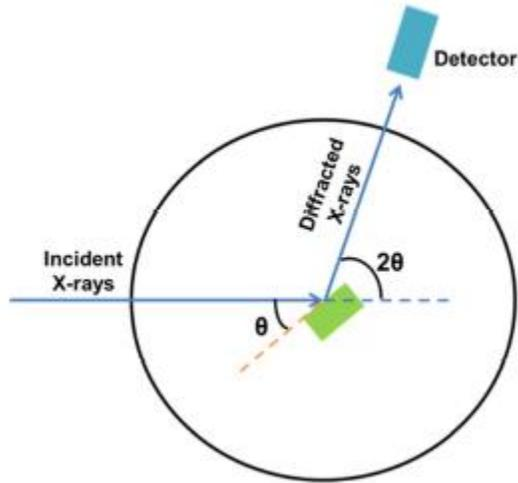
**Figure 3.1.** Representation of typical X-Ray Diffraction[34]
