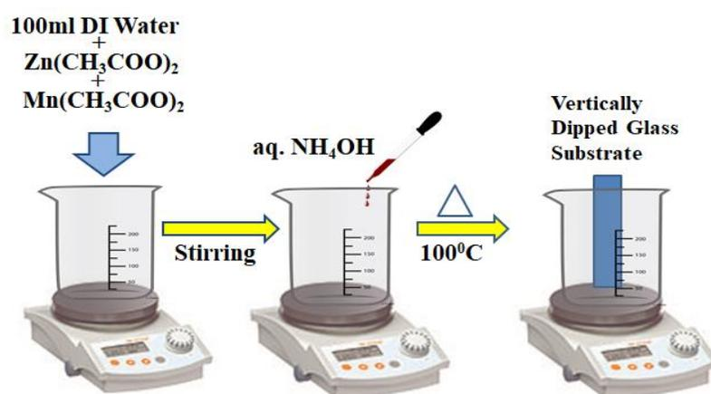
**Figure 4.2.** Synthesis process involved in the material synthesis.
