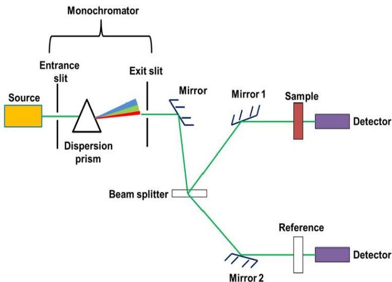
**Figure 3.5.** Experimental setup of UV Vis spectroscopy[34]
