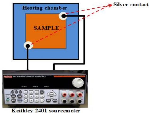
**Figure 6.4.** Experimental setup for the temperature sensor.
