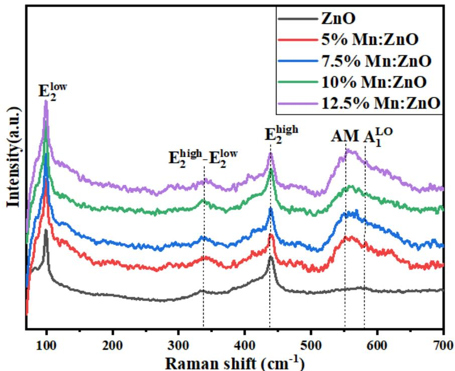
**Figure 5.6.** Raman Spectra of Mn doped and Undoped ZnO.
