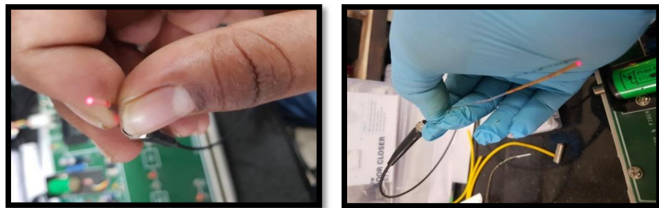
Fig. 29 Light Transmission via Coated Optic Fiber
