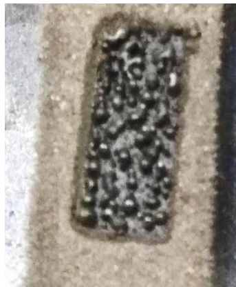
Figure26: Texturing At P=20 W and SS=0.30mm/sec, n=1
