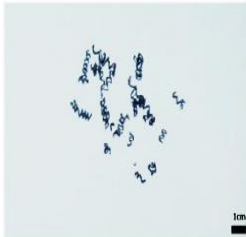
Figure34(a): chip Size at V = 30 \text{ m/min} , f = 0.14 \text{ mm/rev} , d = 0.5 \text{ mm}
