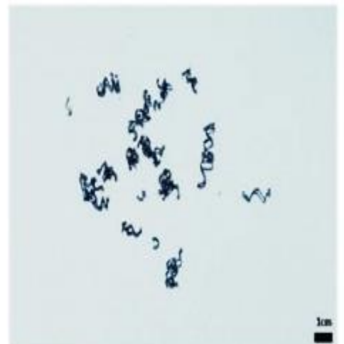
Figure34(a): chip Size at V = 30 \text{ m/min} , f = 0.14 \text{ mm/rev} , d = 0.5 \text{ mm}
