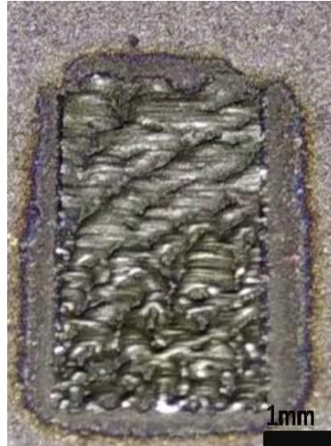
Figure20: SLM of Ni at P=45\text{W} , SS=0.30\text{mm/sec} , n=1
