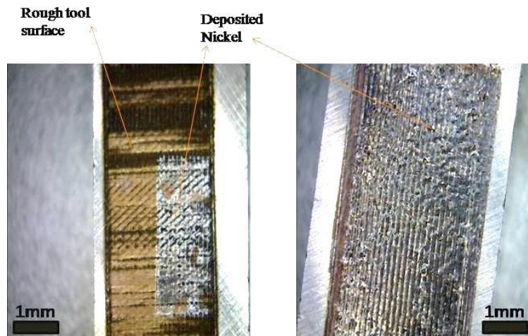
Figure27: Deposited Ni on the tool surface
