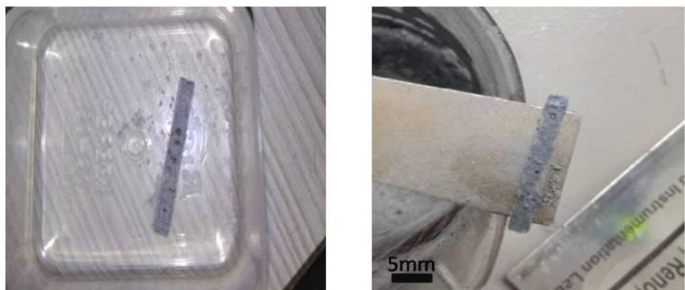
Fig14: SLM of Al at P =15W , SS =0.15\text{mm/sec} , n=5
