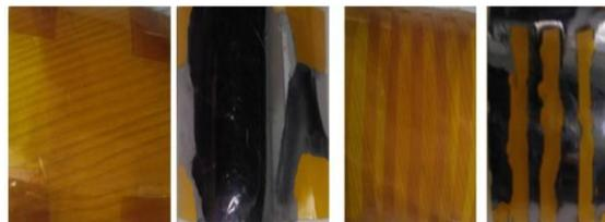
**Fig 11:** Images of patterned SMA created by using Kapton polyimide as a
