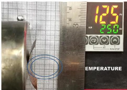
**Fig. 34:** Images of Plate Heating Setup for measuring Shape Recovery
