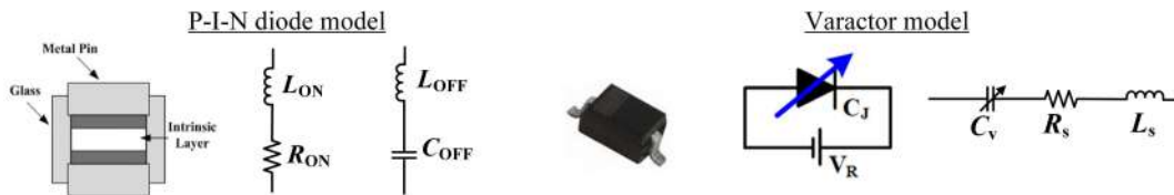
Figure 1.3: Equivalent circuit models of p–i–n diode in the ON and OFF states and varactor diode illustrating voltage-controlled junction capacitance.
