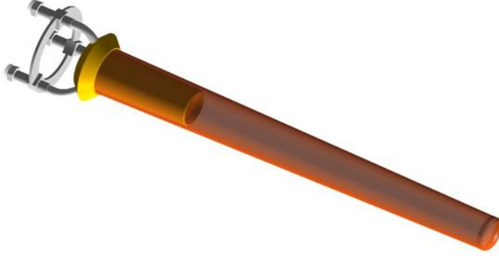
Figure 2.7: The target cell used for the g12 run. Image Source: [36]
