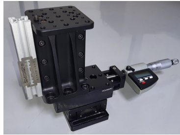
Figure 3.11: Knife Edge translation stage used for beam profiling
