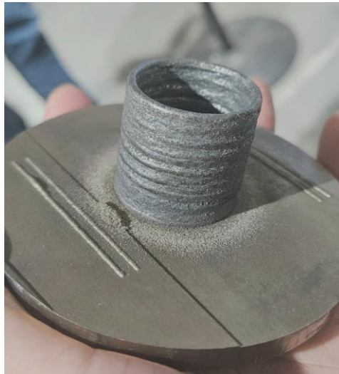
Figure 5.14: First deposition trail of Stellite-21 on R3 powder. The control Algorithm behaved as expected and kept the temperature deviations under control.
