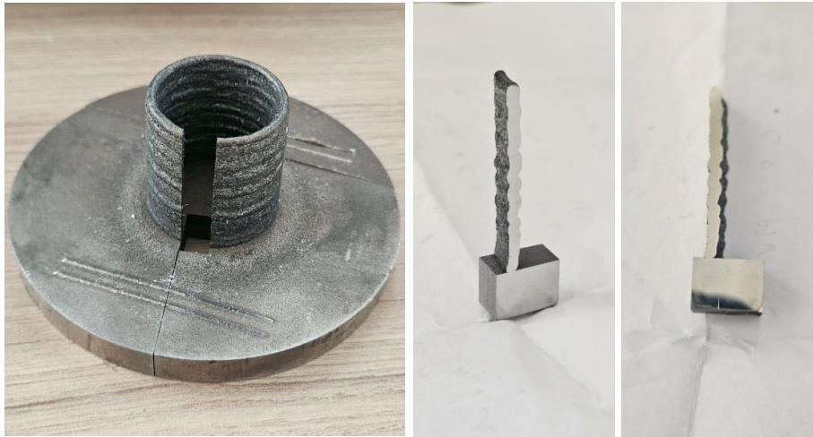
Figure 5.19 : Sample cutting methodology for Hardness Testing across Stellite-21 build layers (Bottom left) sample after being cut (bottom right) Cut and polished sample across Stellite-21 multilayer build height
