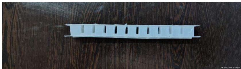
Fig. 5.6: Assembled soft pneumatic actuator after bonding the upper chamber part and the inextensible base layer, showing the complete 11-chamber structure. The single air inlet port is visible at one end.
