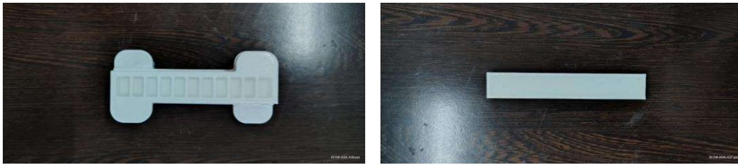
Fig. 5.4 (Left): Cured upper silicone part (upper mold cavity) after demolding, showing the 11-chamber pattern with well-defined chamber geometry and smooth surfaces. Fig. 5.5 (Right): Cured base layer (lower part) after demolding, showing the flat inextensible-reinforced silicone plate.
