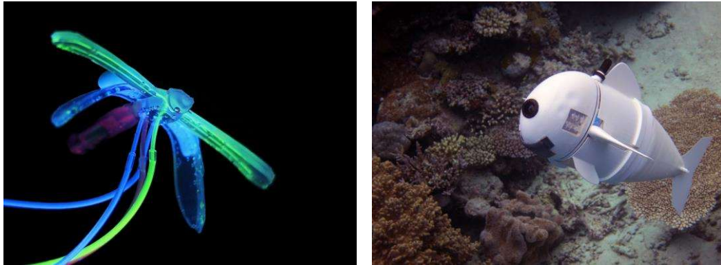
Fig. 1.3 (Left): DraBot, Duke University — a dragonfly-inspired soft robotic platform with pneumatically actuated wings capable of steering through fluid environments. Fig. 1.4 (Right): SoFi, MIT — an underwater soft robotic fish that mimics the undulatory locomotion of biological fish using a soft pneumatic tail actuator. (Image Credit: robotics24.net)
