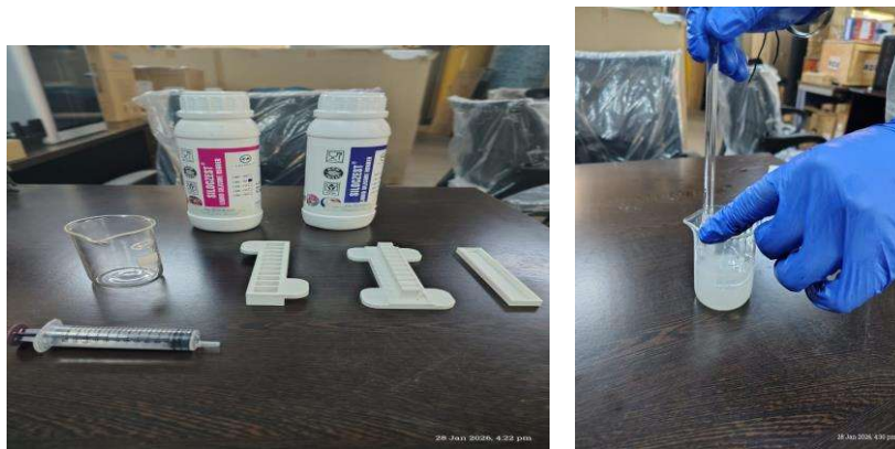
Fig. 5.2 (Left): Preparation stage — Silicozest Part A and Part B bottles, a glass beaker, a syringe for air channel formation, and the PLA-printed mold components arranged on the laboratory bench. Fig. 5.3 (Right): Mixing stage — the Silicozest A+B mixture being stirred slowly with a glass rod in the beaker prior to pouring into the molds.
