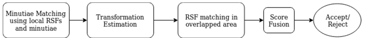
Fig. 3.6 Matching algorithm flowchart
