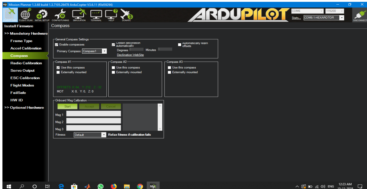
Fig2.23: Compass Calibration in Mission Planner
