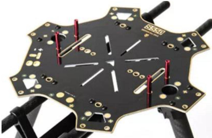
Fig2.13(b): Integrated power distribution board for hexa-copter
