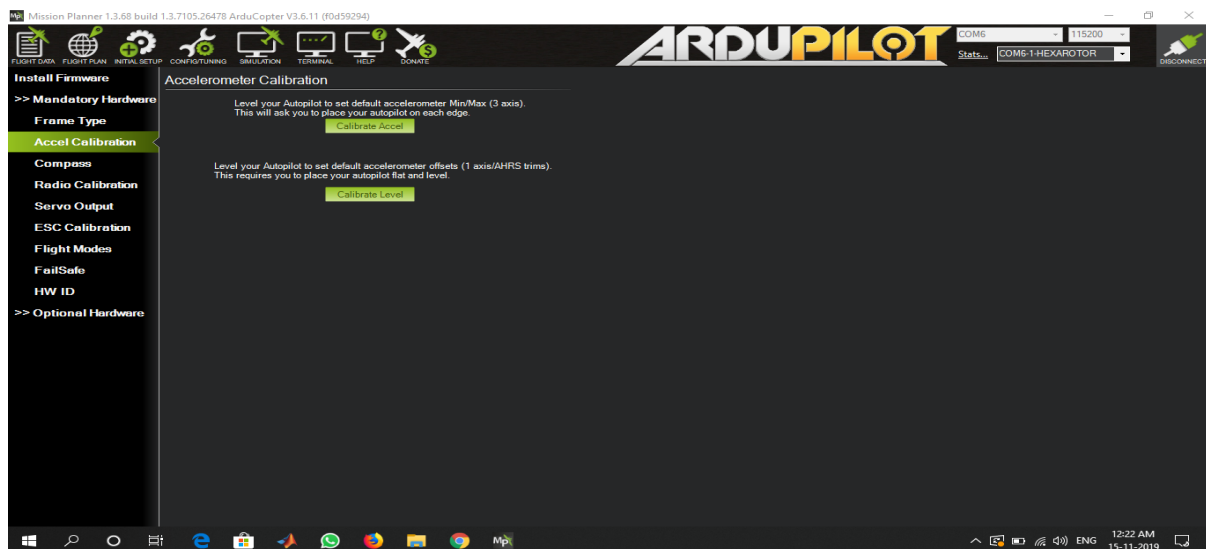
Fig2.22: Accel Calibration in Mission Planner
