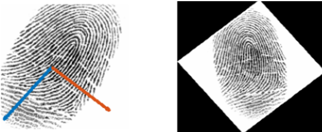
Figure 3.6: PCA applied on the right aligned image
