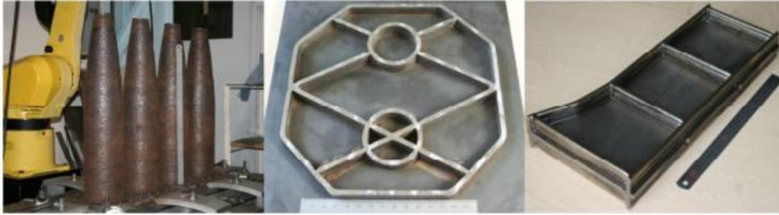
Figure 1-1 : Components built by the WAAM process: (a) shell castings; (b) part with crossovers and intersections; (c) Ti aerospace component.
