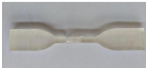
***Fig 23:Specimen after failure***
