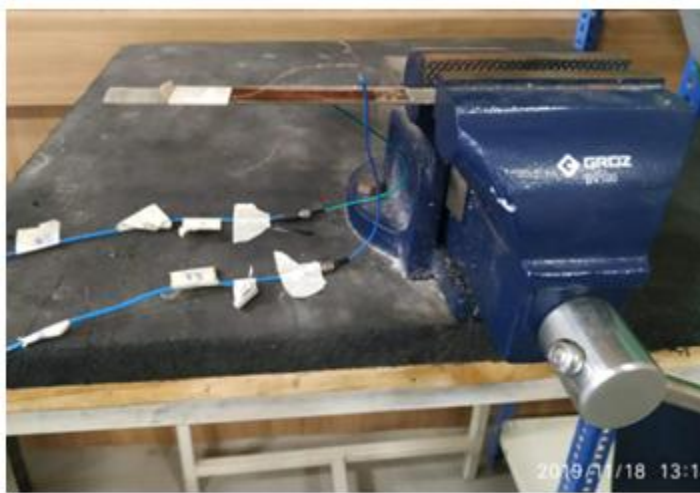
Fig.20 - Experimental setup: (i) PVEH beam connected to data acquisition system; (ii) NVGate software used to generate the FRF
