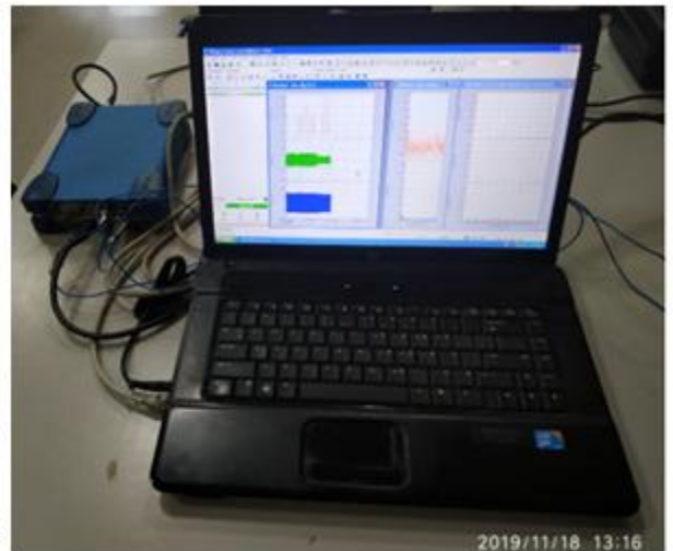
Fig.20 - Experimental setup: (i) PVEH beam connected to data acquisition system; (ii) NVGate software used to generate the FRF
