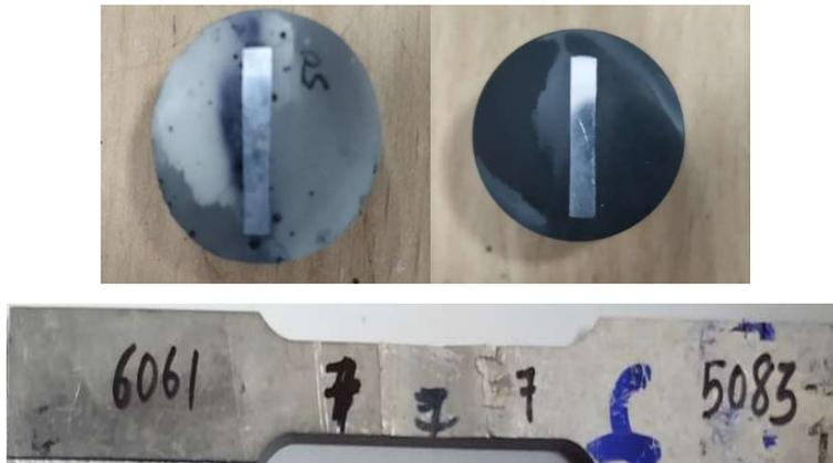
*Figure 6. Sample preparation, (a) cold mounting, (b) hot mounting and (c) tensile specimen.*
