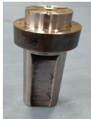
Figure 16. Tool design used for FSPAM
