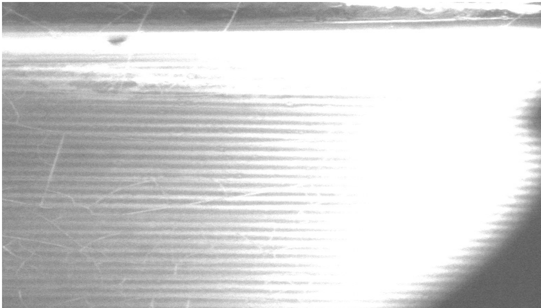
Figure 5: Line patterns of 10 lp/mm Ronchi grating superimposed on cuvette.
