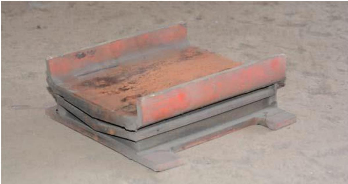
Fig 3.2. Elastomeric pad [5]
