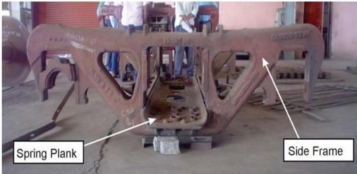
Fig 3.4 Side frame and spring plank [5]
