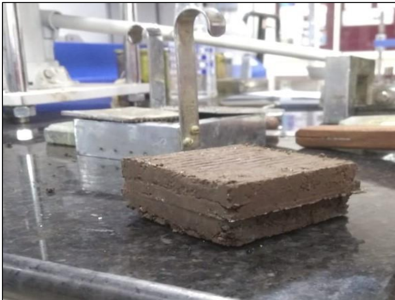
Fig.6 (b). Shear sample of black cotton soil mixed with 5% fly ash at 100kPa normal loading and 0.25mm/min. strain rate.
