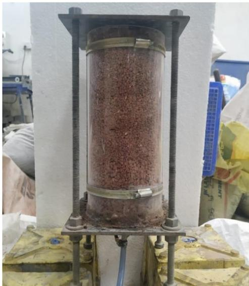
Fig.6: Injection test apparatus filled with dry crushed bricks
