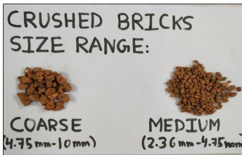
Fig.1: Two different size ranges of crushed bricks.
