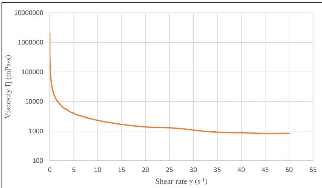
Fig.11: w/c 0.45 viscosity curve for down-ramp
