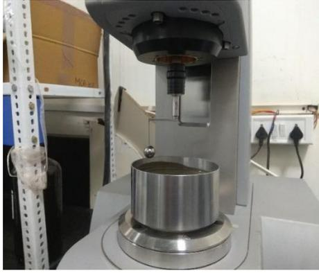
Fig.4: Rheometer apparatus along with BM-15 ball and grout sample
