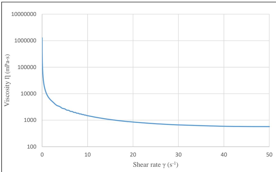
Fig.15: w/c 0.55 viscosity curve for down-ramp
