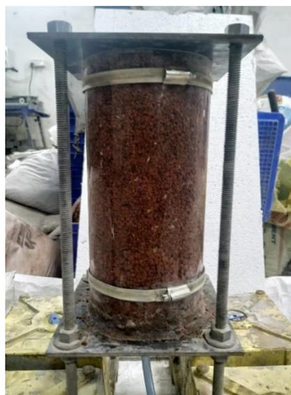
Fig.7: Injection test apparatus with pre-wet crushed bricks
