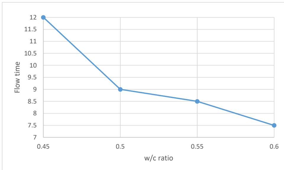
Fig.8: Flow time vs. w/c ratio
