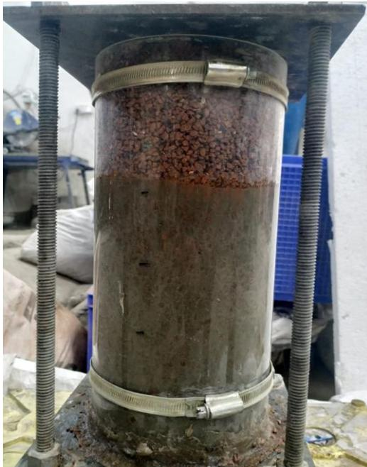
Fig. 19: PM injected with w/c 0.60 grout
