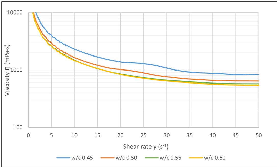
Fig.23: Comparison of viscosity curves of cement grouts
