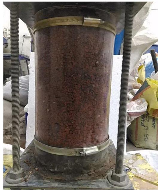
Fig. 21: PM injected with w/c 0.50 grout      Fig. 22: PM injected with w/c 0.45 grout
