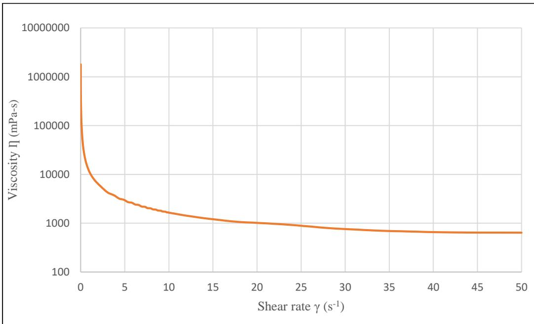
Fig.13: w/c 0.50 viscosity curve for down-ramp
