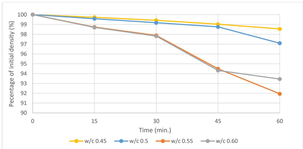
Fig. 9: Variation of the density of grout mixes with respect to time
