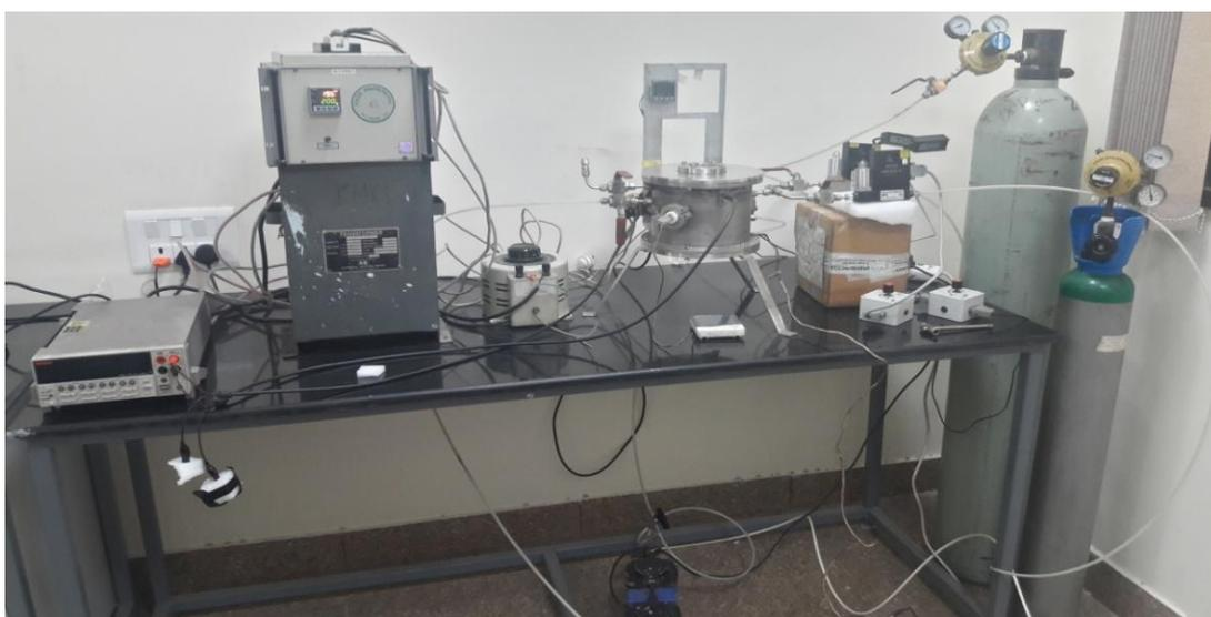
**Figure 4.4: Gas Sensing Setup used for CO Sensing Analysis.**
