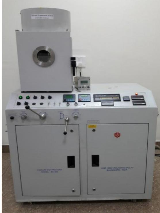
**Figure 3.1: Thermal Evaporation System used for Cu Thin Film Deposition.**
