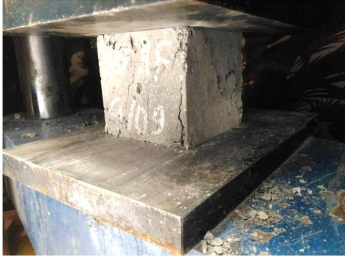
Figure 8 Compressive strength test on concrete
