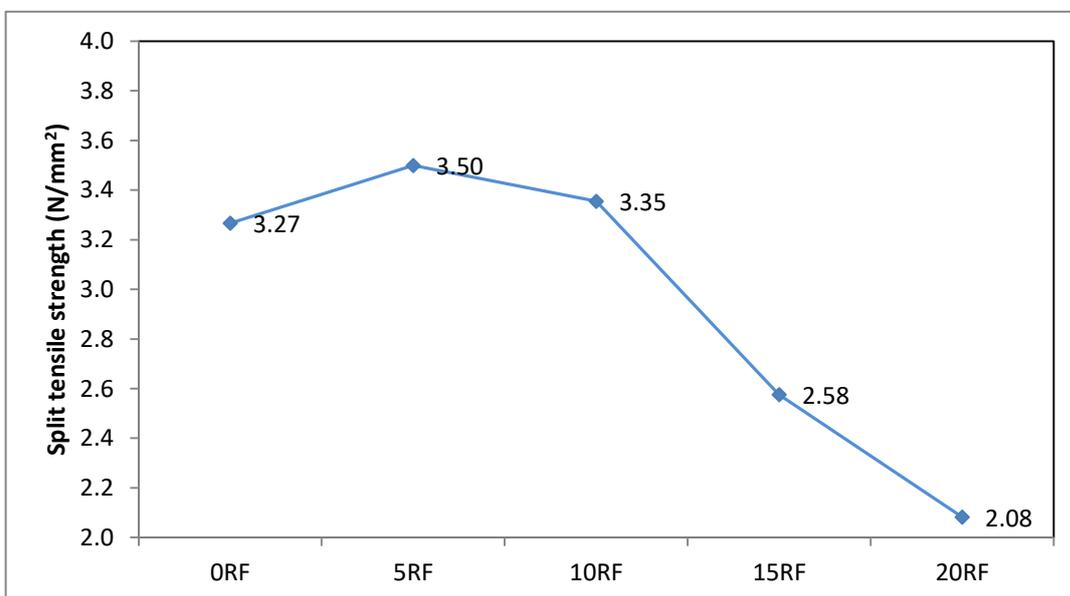
Figure 16 Split tensile strength test results
