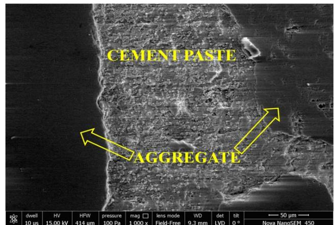
Figure 20 Microstructure of 0RF at 1000x zoom
