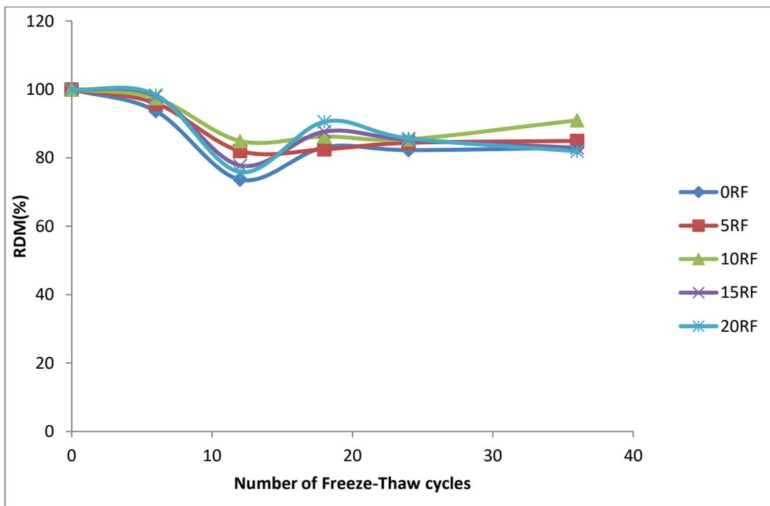
Figure 13. Relative Dynamic modulus of concrete mixes with increasing Freeze-thaw cycles
