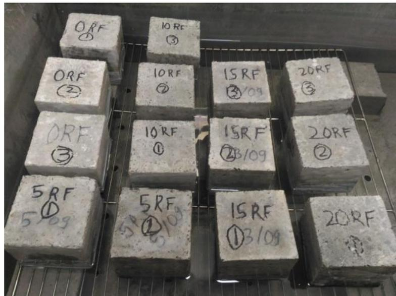
Figure 11 Capillary water absorption test
