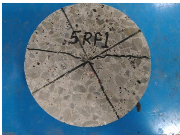
Figure 14 Impact Failure
