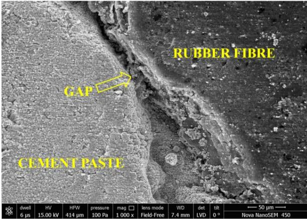
Figure 21 Microstructure of 5RF at 1000x zoom
