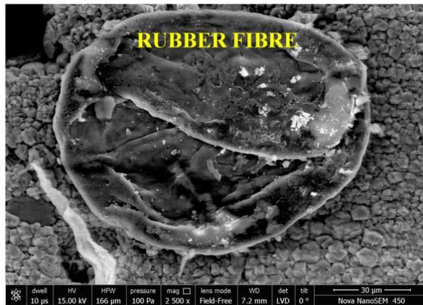
Figure 25 Microstructure of rubber fiber crosssection at 2500x zoom
