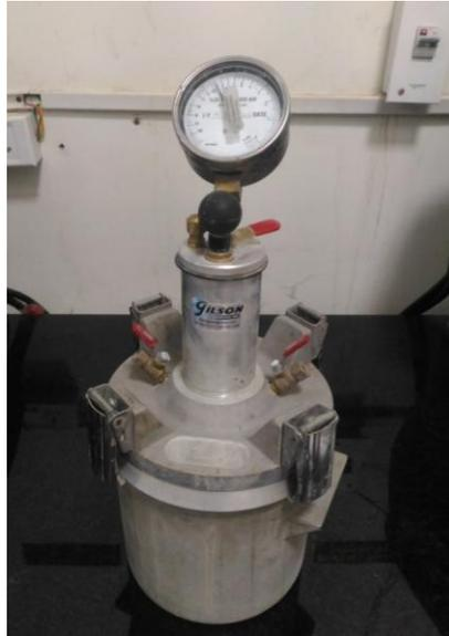
Figure 4 Test apparatus for air content in concrete
