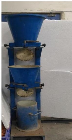
Figure 3 Compaction factor test set-up
