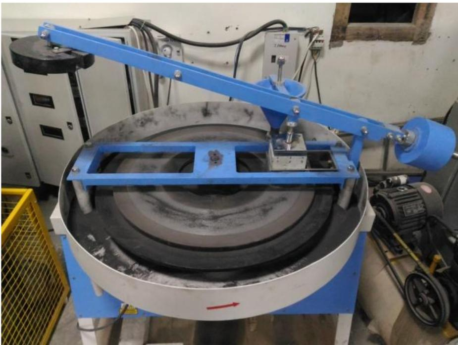
Figure 10 Abrasion test on concrete specimen
