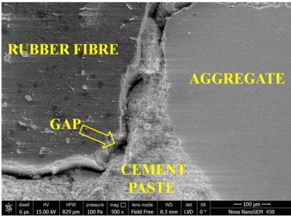
Figure 23 Microstructure of 15RF at 500x zoom
