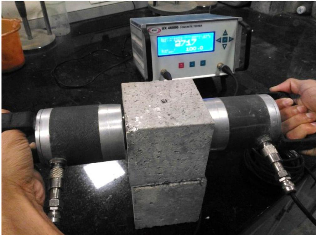
Figure 7 UPV on the concrete specimen
