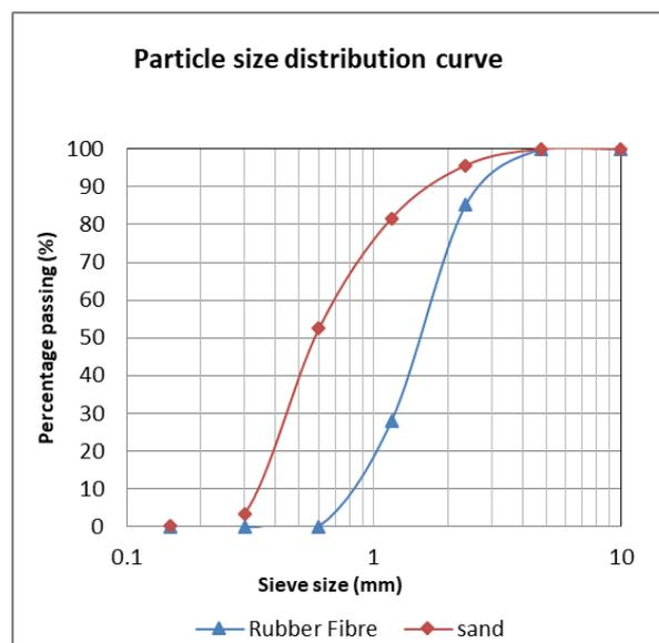
Figure 2 Particle size distribution of fine aggregates and rubber fiber
