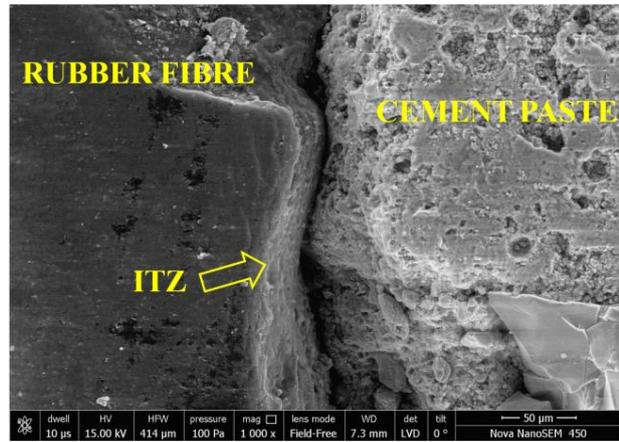
Figure 24 Microstructure of 20RF at 1000x zoom
