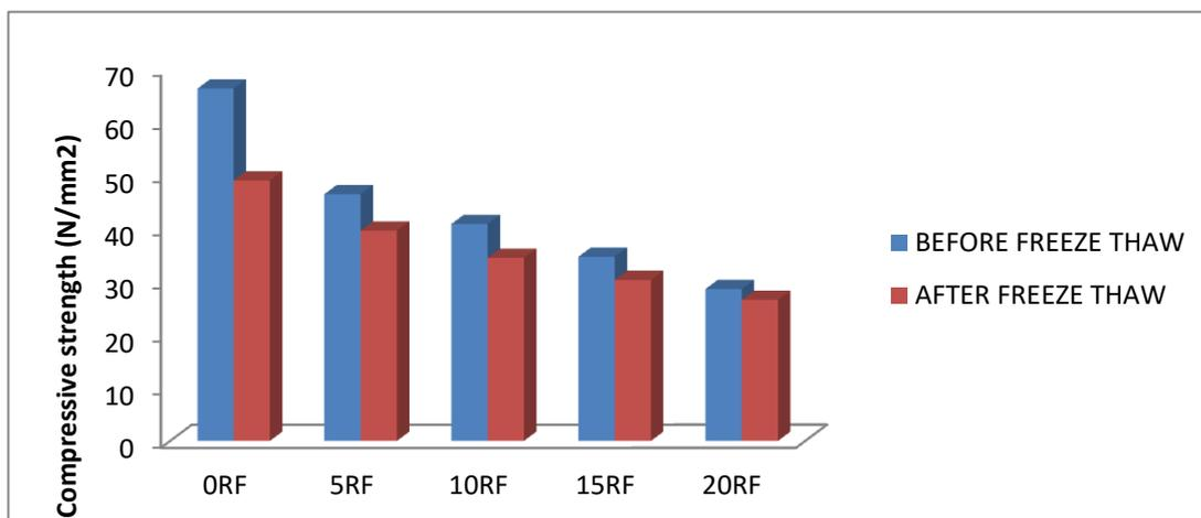
Figure 12 Compressive strength of concrete mixes before and after 36 Freeze-Thaw cycles
