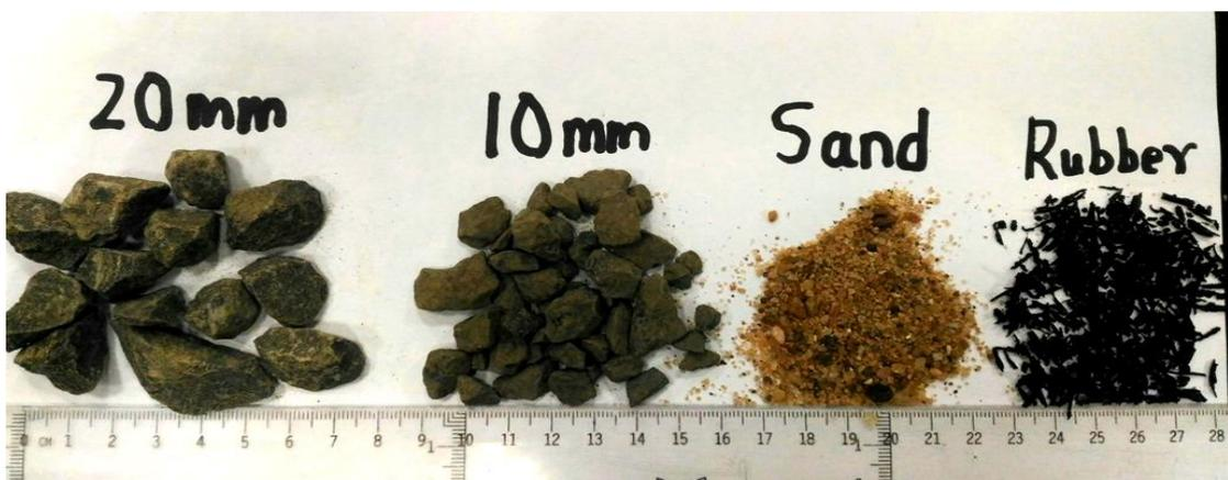
Figure 1 Raw materials used as concrete ingredients
