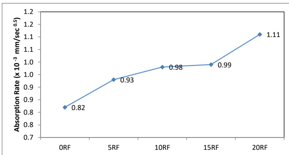
Figure 18 Capillary water absorption test results
