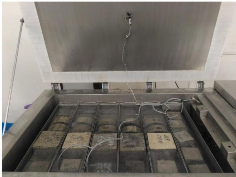
Figure 6 Arrangement for freeze and thaw test on concrete
