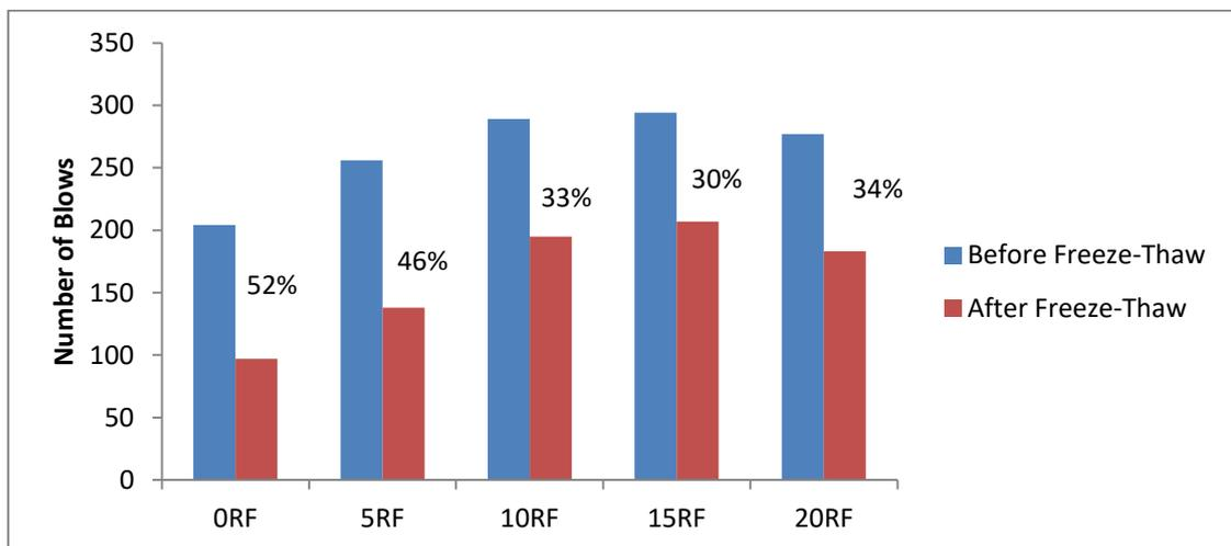
Figure 15 Impact Resistance of concrete mixes
