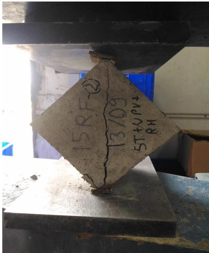
Figure 9 Set-up of split tensile strength test
