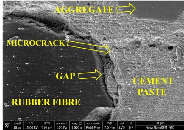
Figure 22 Microstructure of 10RF at 1000x zoom
