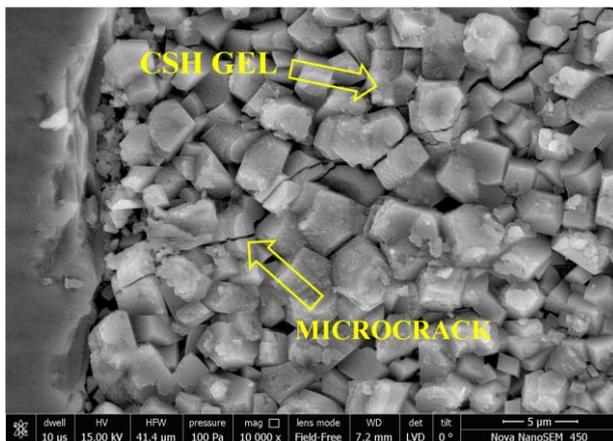
Figure 19 Microstructure of 0RF at 10000x zoom
