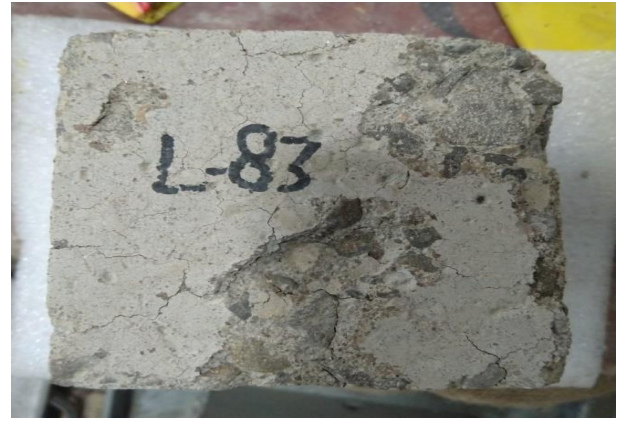
b. Sample after subjecting to 1000 °C for 4 h.
