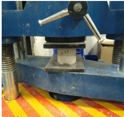
Figure 4. The sample placed between the upper and lower plate of UTM
