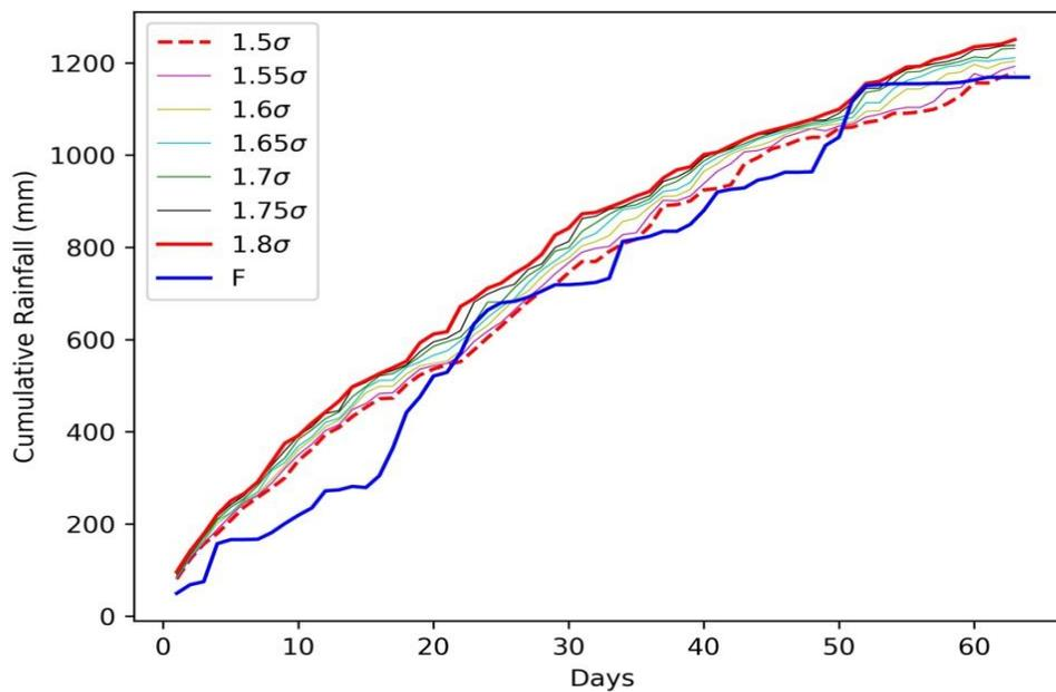
Figure 10 Visualization of calibration algorithm. The threshold value was raised till the cumulative rainfall curve of the event (F) is not crossing the threshold curve. (Standard Threshold of 1.75 is optimized to 1.80)
