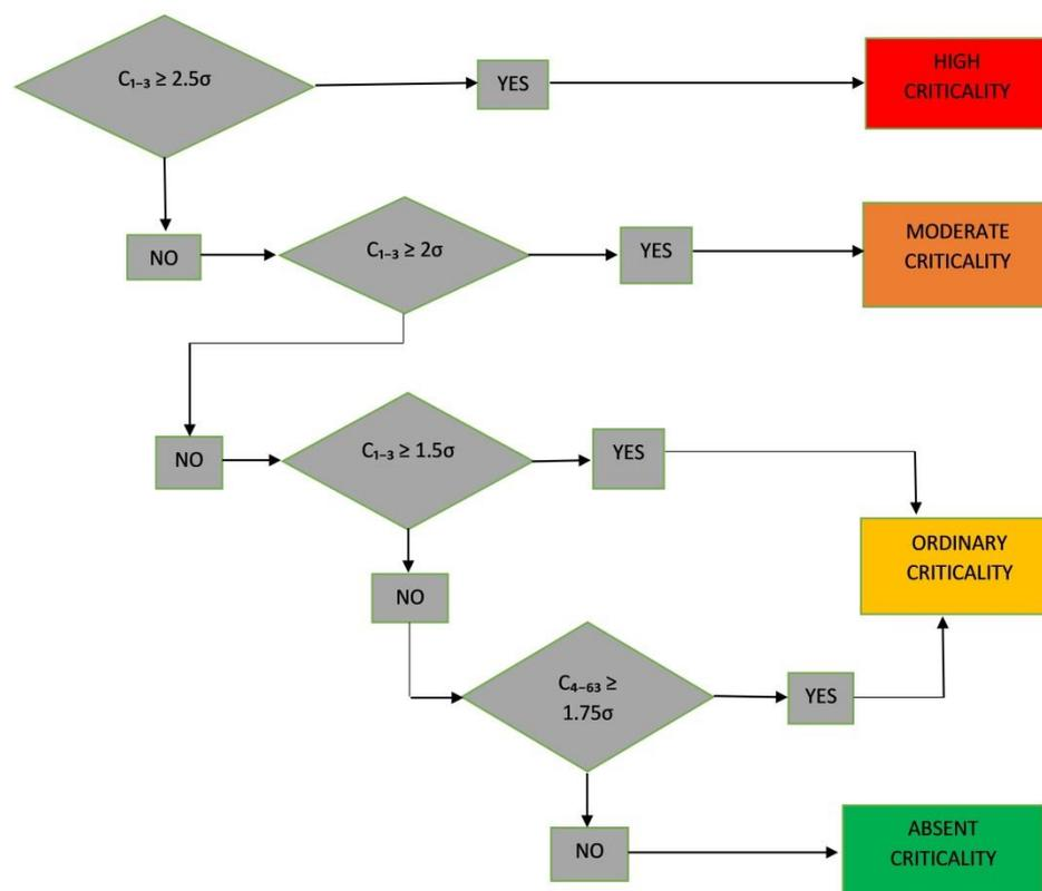
Figure 9 Algorithm used for calibration of the SIGMA model for Kalimpong town.
