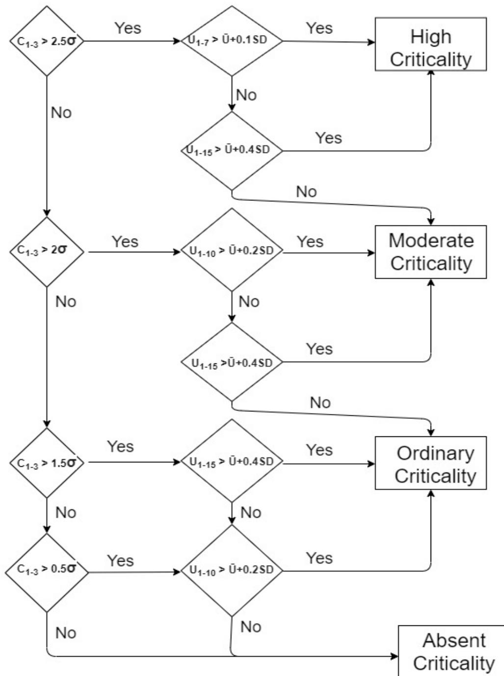
Figure 13 Scheme of the SIGMA-U algorithm.  $C$  is cumulative rainfall,  $U$  is soil moisture,  $\bar{u}$  is average soil moisture and  $SD$  is standard deviation of soil moisture series.
