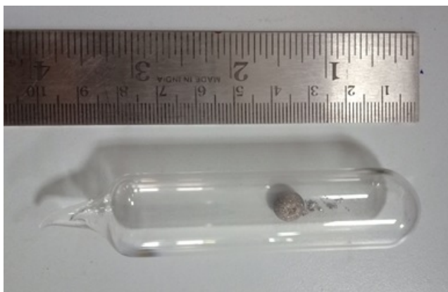
Figure 2.2: A quartz ampoule with a sample bead inside. A measuring scale is placed to indicate the size of the ampoule.
