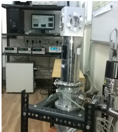
Figure 8.1: Resistivity measurement probe with a standard sample mounted on it.
